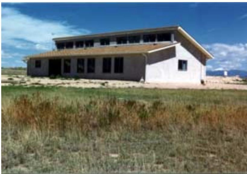
Figure 6. Overhangs shading south glazing in summer
