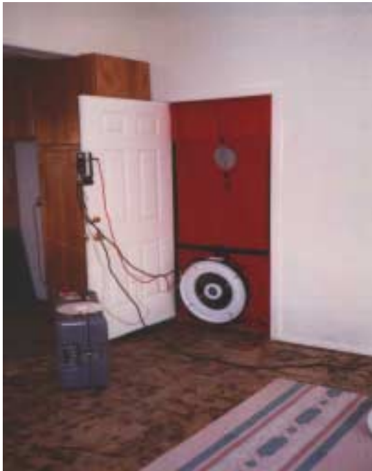
Figure 14. Blower door test setup
