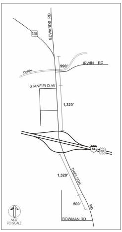
• The Bowman Road/Thielsen Road intersection is located approximately 2,300 feet south of the interchange. Based on the existing spacing from the interchange, this intersection is an ideal location for an additional full access intersection on Thielsen Road. The Bowman Road/
