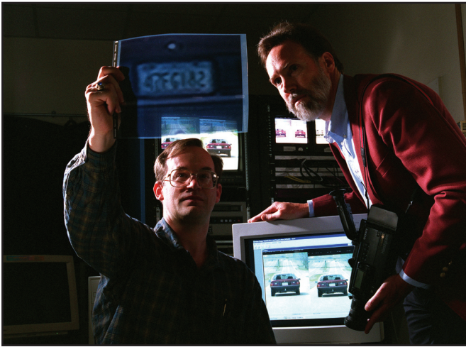
NASA inventors Paul Meyer, left, and Dr. David Hathaway view a license plate number revealed by using the Video Image Stabilization and Registration -- VISAR -- software to improve poor quality footage.
