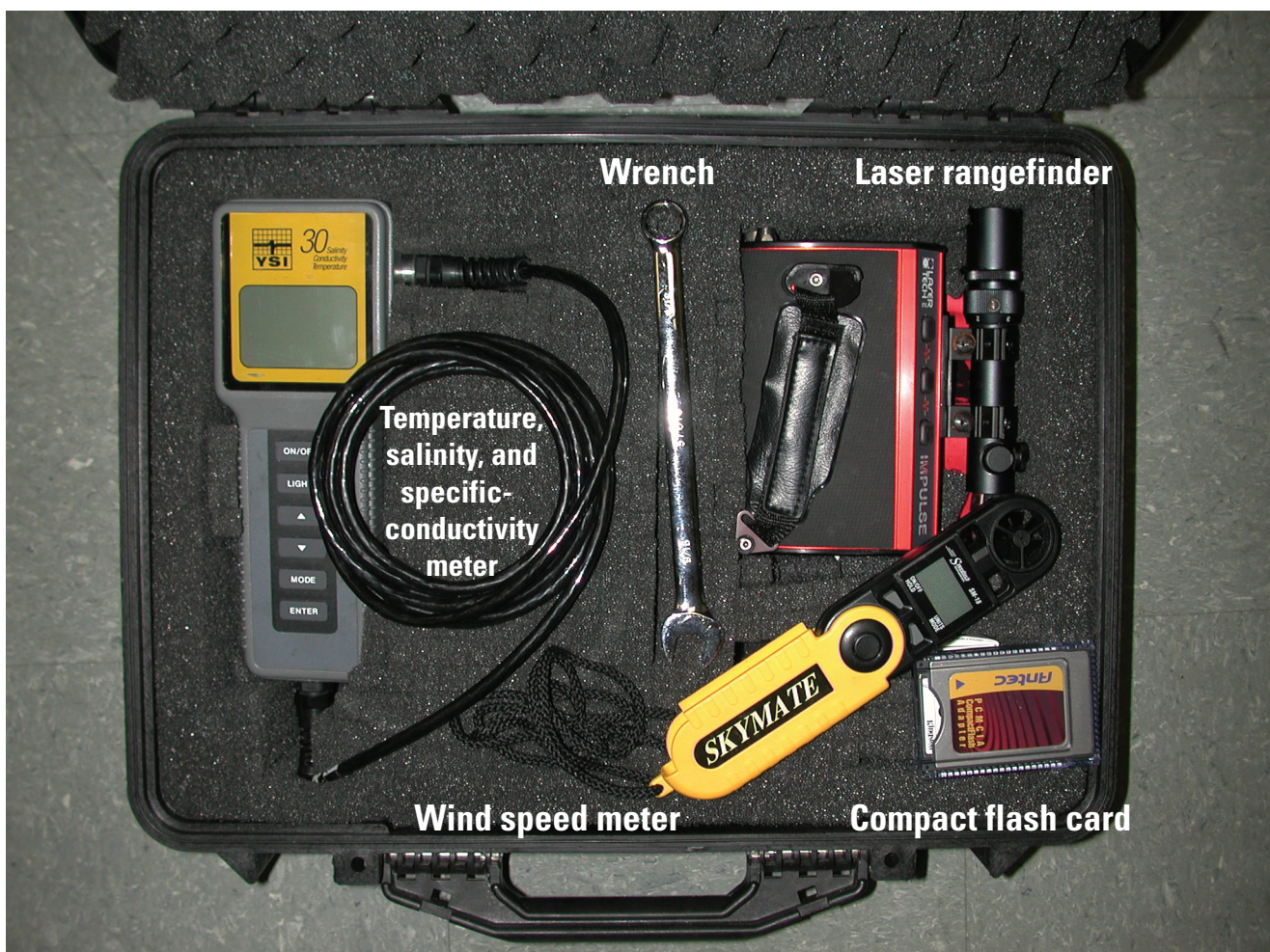
Figure 2. Example toolkit of ancillary equipment for use with acoustic Doppler current profilers (ADCPs) when making streamflow measurements. (Photograph by John M. Shelton, U.S. Geological Survey.)
