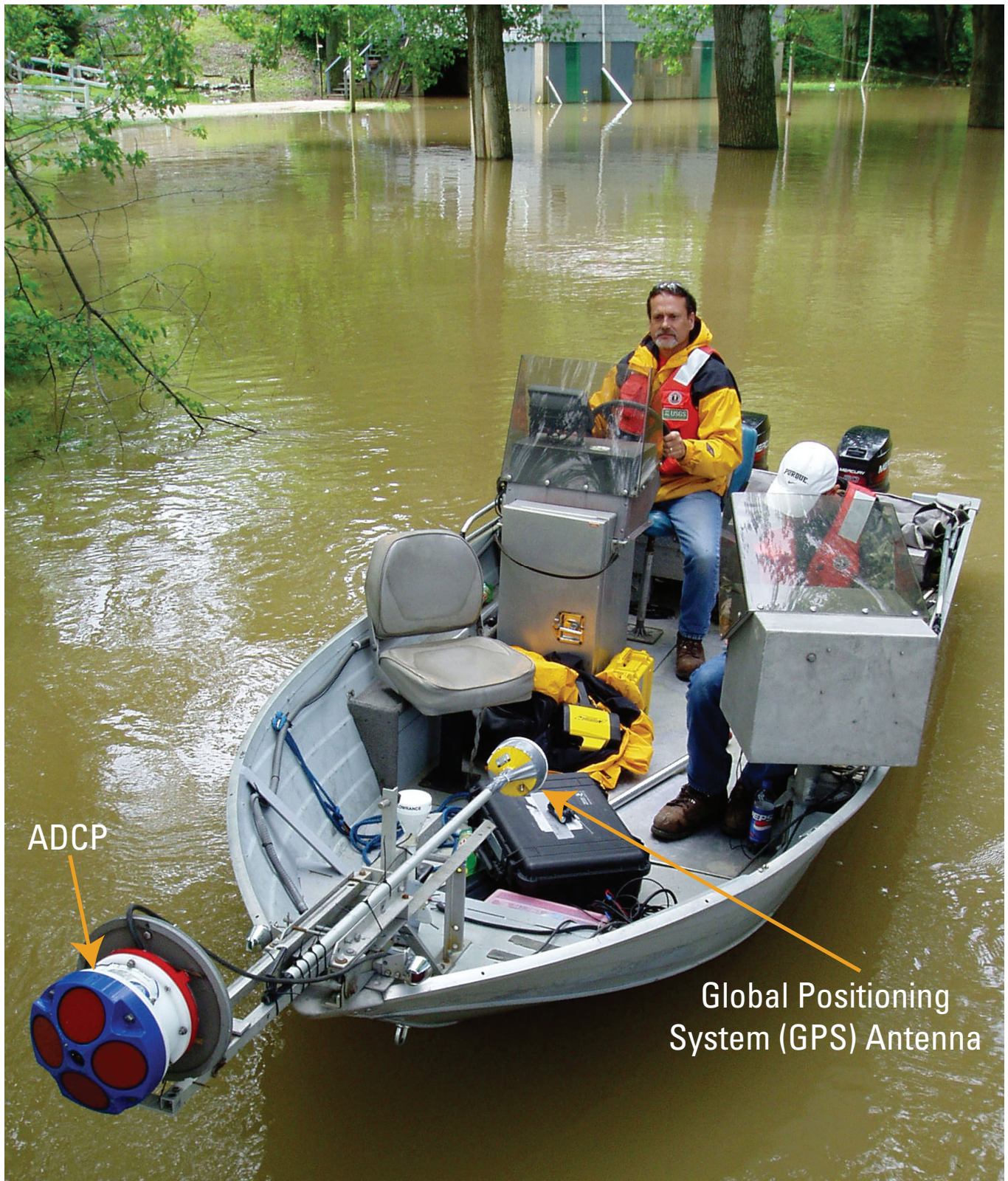
Figure 4. Bow-mounted acoustic Doppler current profiler (ADCP) mounting brackets and ADCP on U.S. Geological Survey work boat. (Photograph by Paul Baker, U.S. Geological Survey.)
