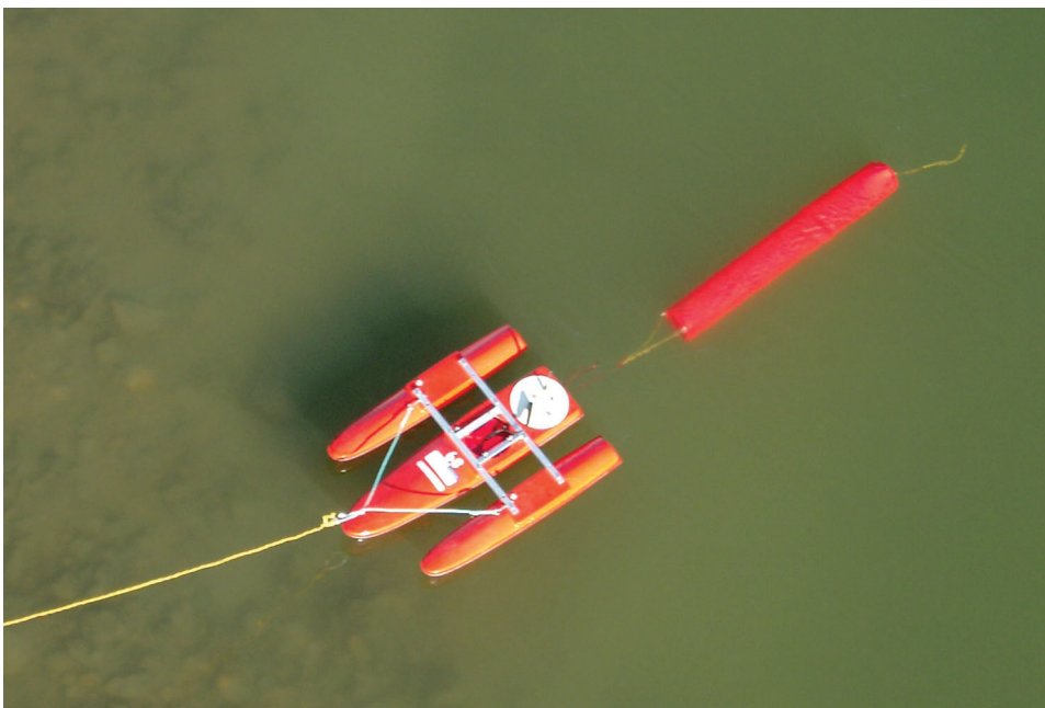
Figure 7. Tethered acoustic Doppler current profiler boat with a sea anchor attached (from Environment Canada, 2004). (Photograph by Clare Bowden, Environment Canada).
