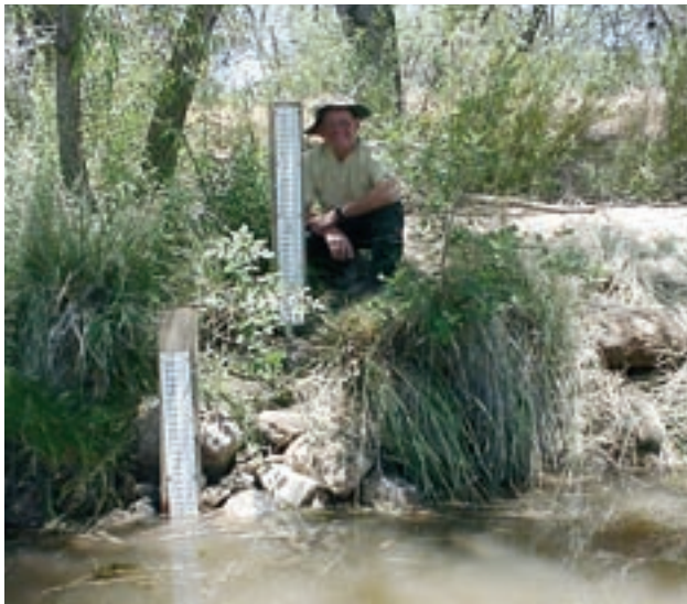
Figure 2. Staff gages at pool in Rincon Creek, Saguaro National Park (NPS, June 2003)
