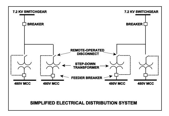
The following remote indications are observed for a 480 VAC load center supply breaker. (The breaker is normally open.)
