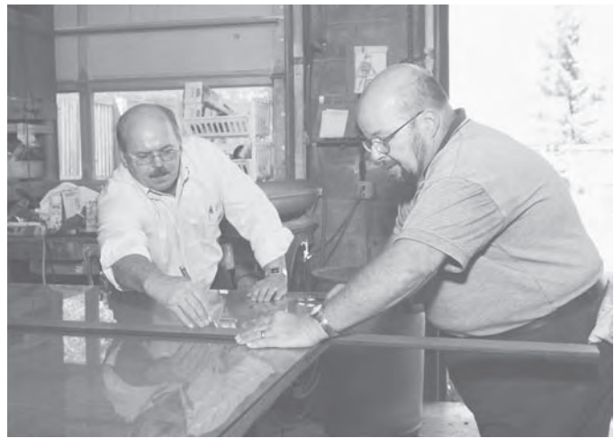
Using a straightedge as a guide, the glazier makes a score on the surface of the glass before cutting it.
