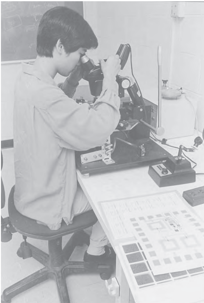
Semiconductor processing technicians use microscopes to check for flaws in semiconductor wafers.
