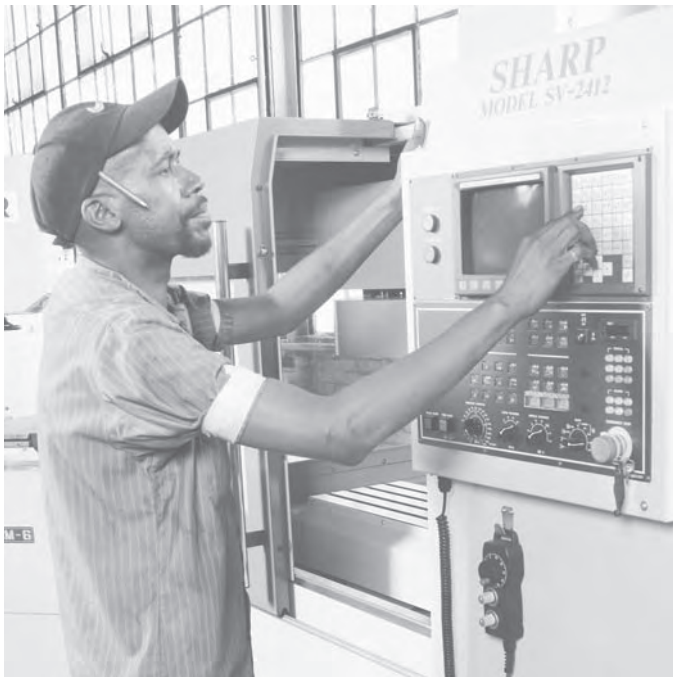
Computer control operators load programs into a machine.
