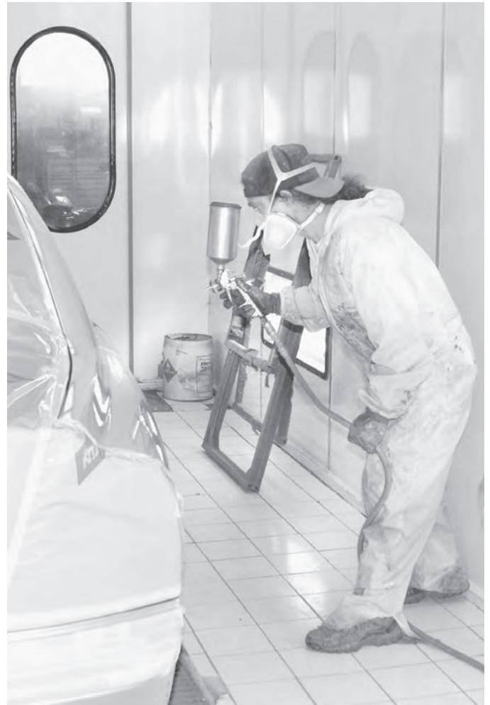
To minimize exposure to harmful chemicals, painting and coating workers must wear protective masks when performing certain tasks.
