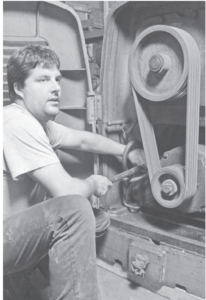
An industrial machinery mechanic adjusts a belt to reduce friction.
