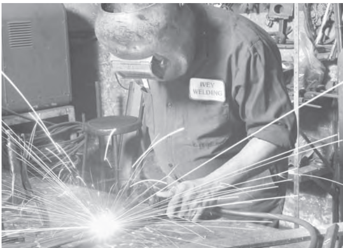
Eye protection is important during arc welding.
