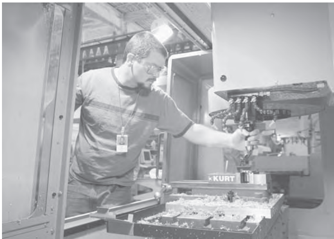
Machinists use computer controlled machine tools to make parts.
