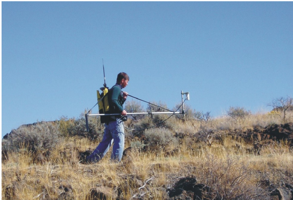
Figure 8. Photo. Data collection with the Geometrics G-858 Magnetometer at LBNM.
