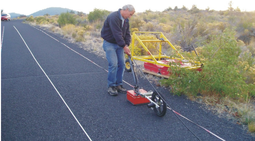
Figure 7. Photo. GPR data collection with the 400 MHz antenna at LBNM.
