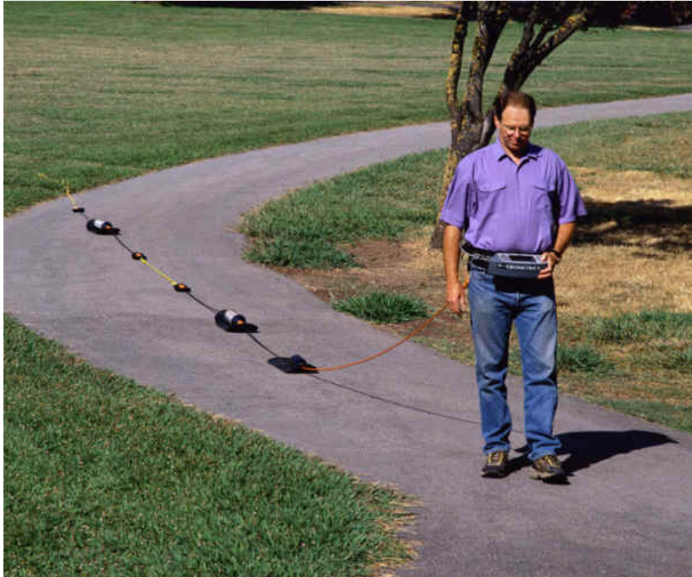
Figure 4. Photo. Data collection with the OhmMapper.
