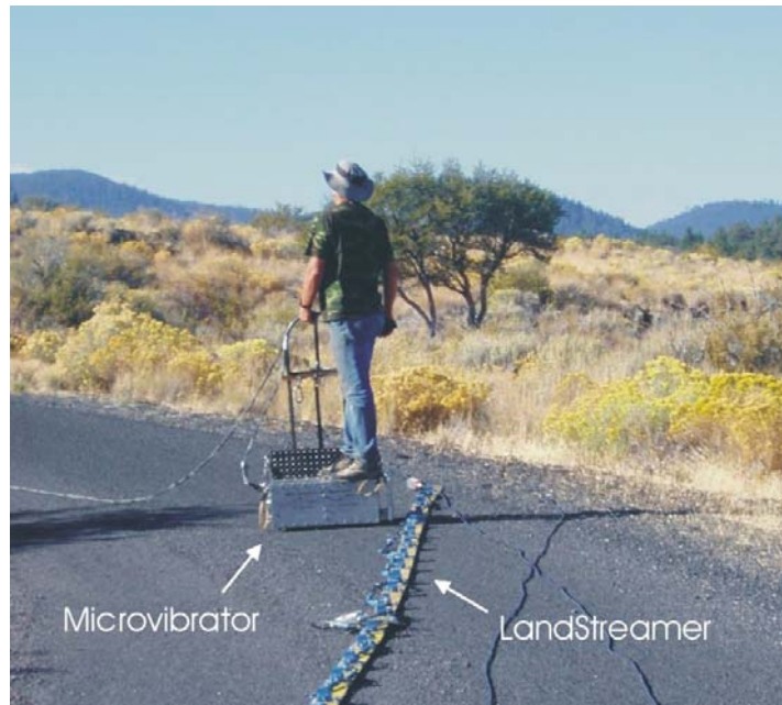
Figure 13. Photo. Data collection with the MicroVibrator and the Land Streamer at LBNM.
