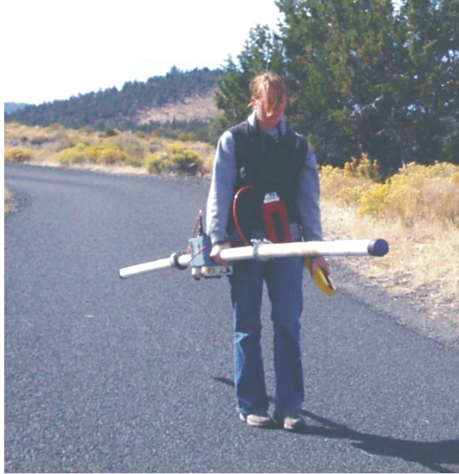
Figure 9. Photo. Data collection with the EM31 at LBNM.
