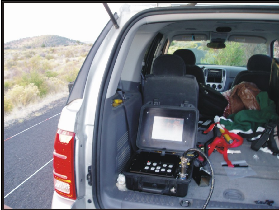
GSSI Sir-2000 Control Unit In Back Of Automobile
