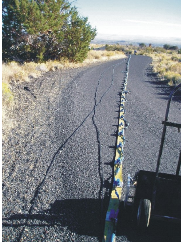
Figure 16. Photo. Land Streamer deployed above Golden Dome Cave.
