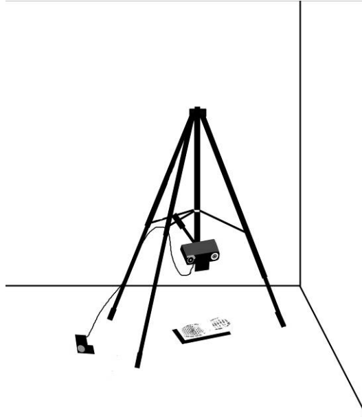
Figure 6: Representation of the camera and tripod setup for shoeprint photography
