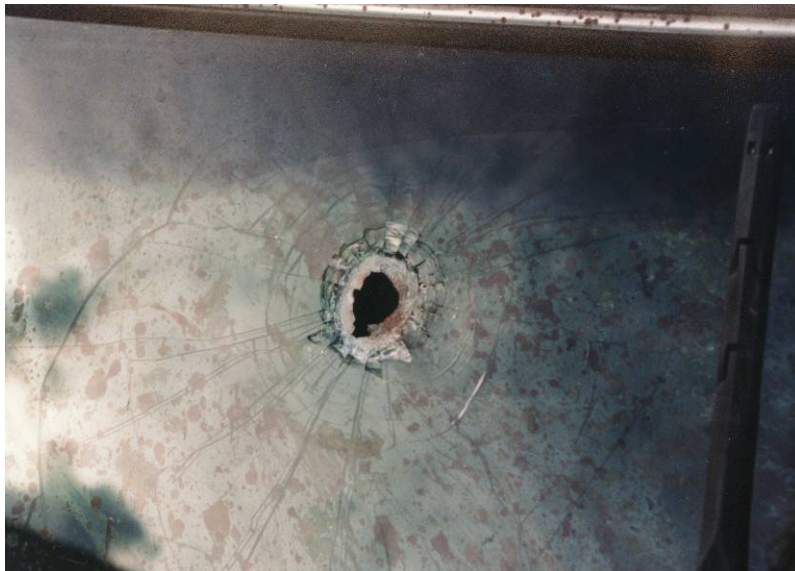
Figure 8: Exterior view of a vehicle windshield with a bullet hole. Examination of the characteristic fracturing around the hole revealed the shot was fired from the inside of the window to the outside, not from outside to inside.
