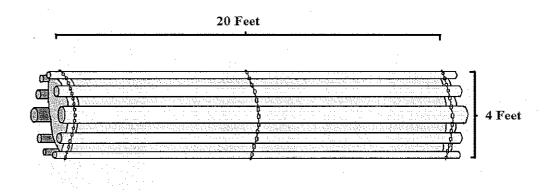
This is not a bundle of smaller logs but a tube of logs that is filled with cobble sized river rock or small boulders and constructed in place.
