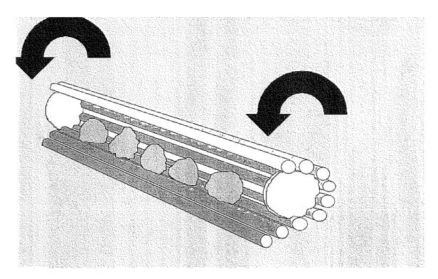
Gabion logs would not be buoyant. In a tidal estuary environment floating LWD does not provide habitat advantages and are hard to maintain in place. Gabion Logs of this type would be tremendously heavy and would not require the cabling in lower velocity flow areas of the estuary or ponded reaches.
