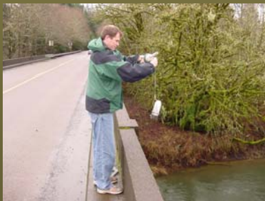
Collecting surface grab samples for monitoring
