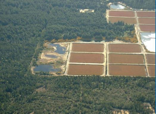
Sea Wind Cranberries is experimenting with artificial wetlands to "scrub" nitrates and phosphates from bed tailwater. Though the wetlands did an excellent job, none of the water entering the wetland from the beds was above standards.
