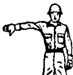
LOWER BOOM AND RAISE LOAD (FLEX FINGERS)
