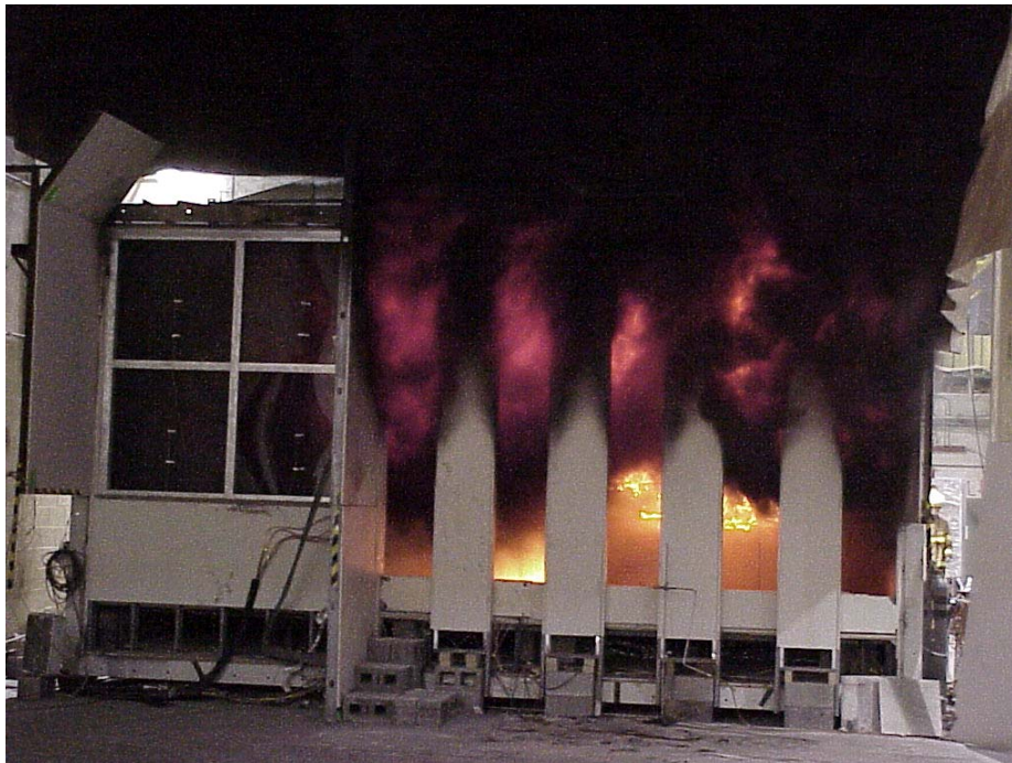
Figure 6–34. Three-workstation fire test, 2 min after the start.
