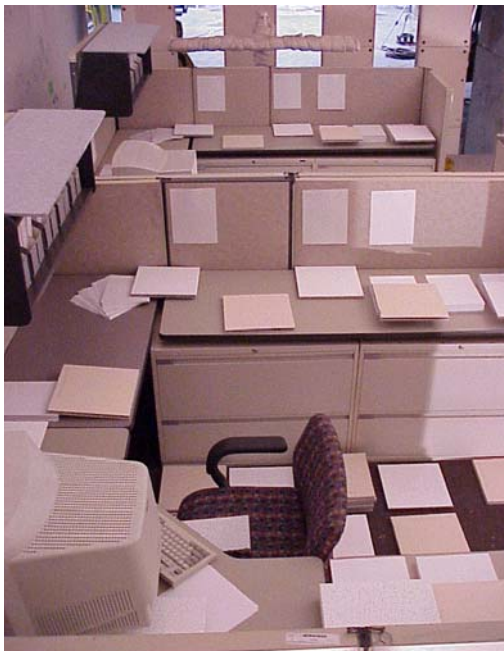
Figure 6–32. Interior view of a three-workstation fire test.
