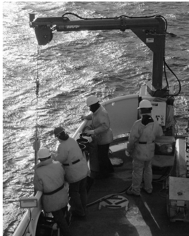
Figure 1. Free-fall cone penetrometer (FFCPT) being deployed with free-fall winch. Photo by Robert McConnaughey.
