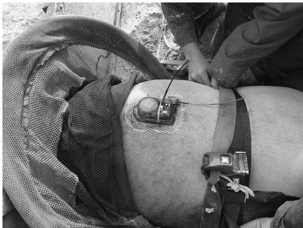
FastLoc global positioning system instrument attached to adult female California sea lion at San Miguel Island, California, November 2005. Photos by Tony Orr.
