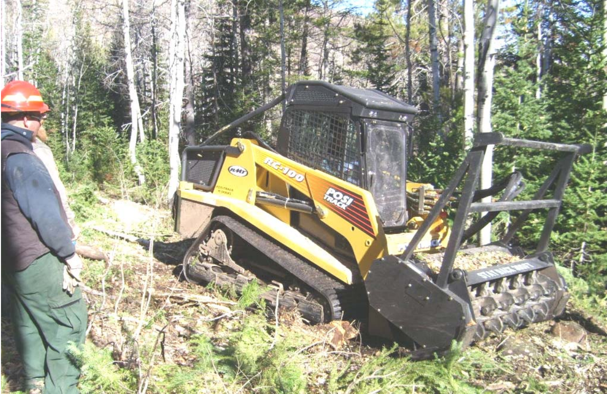
Photo above: A “skid steer” with attachment head operating in an aspen/conifer stand.
