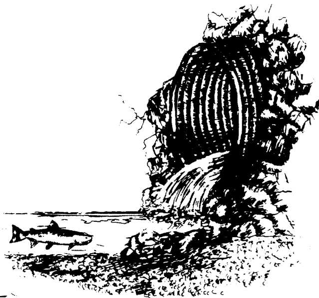
No resting pool below culvert
