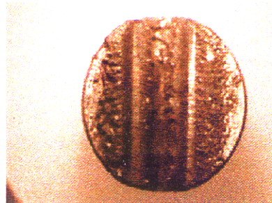
Aluminum V-block After Falex test with SW220-Proateq and R-134a
