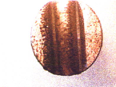
Aluminum V-block After Falex test with York C-Proateq and R-22
