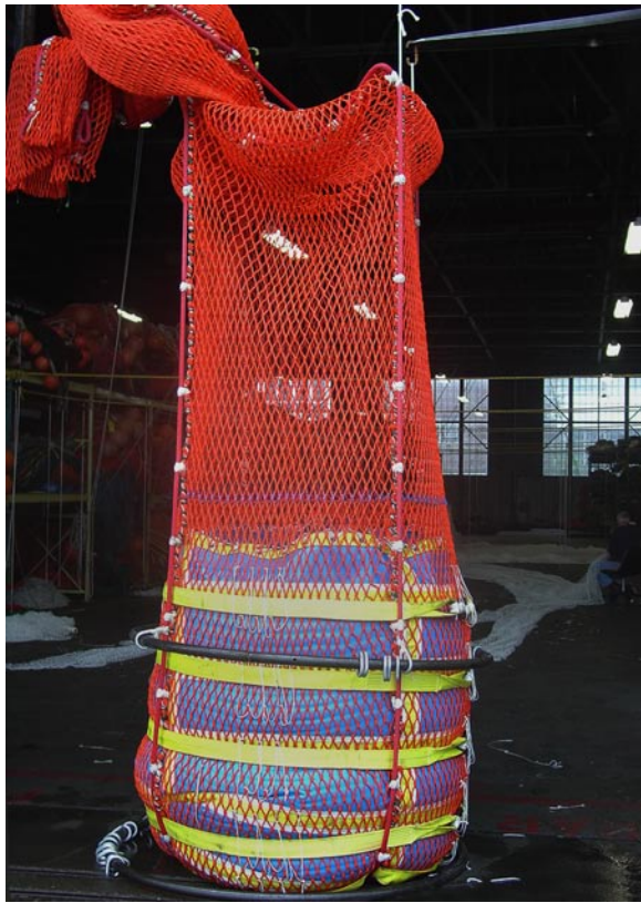
Figure 1. Prototype net for sampling walleye pollock for future tagging experiments. Photo by David King.
