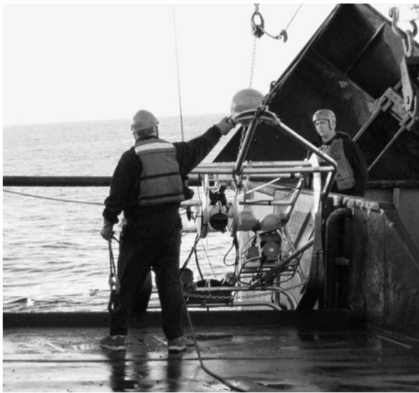
Figure 2. Launching the seafloor sled with DIDSON sonar and camera with strobed lighting. Photo by Carwyn Hammond.
