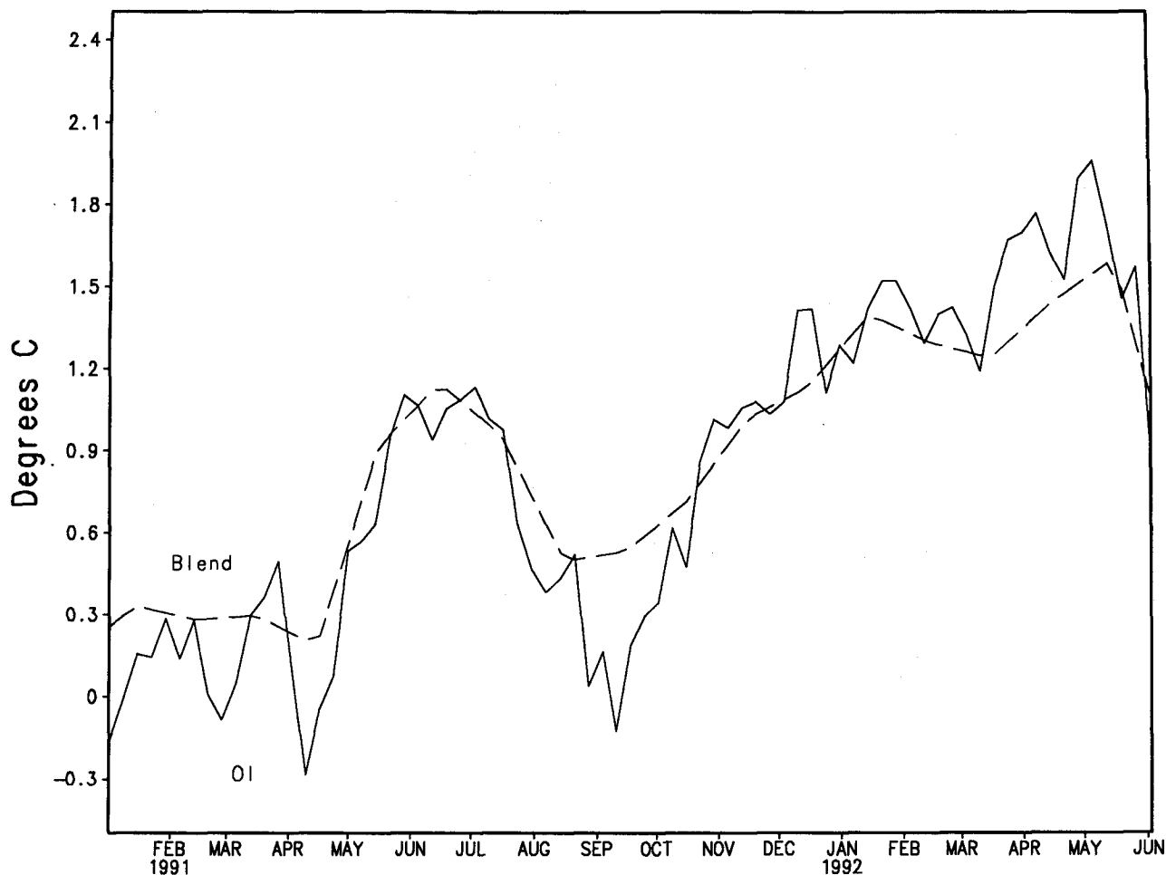
FIG. 19. Average SST anomalies from the blend and the OI with the satellite bias correction for the Niño 3 area: 5°S–5°N, 150°W–90°W.
