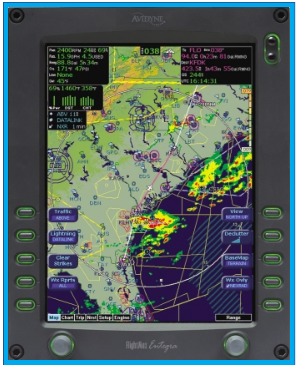
Avidyne® Entegra MFD offers many features including weather overlay. (Avidyne® photo)
