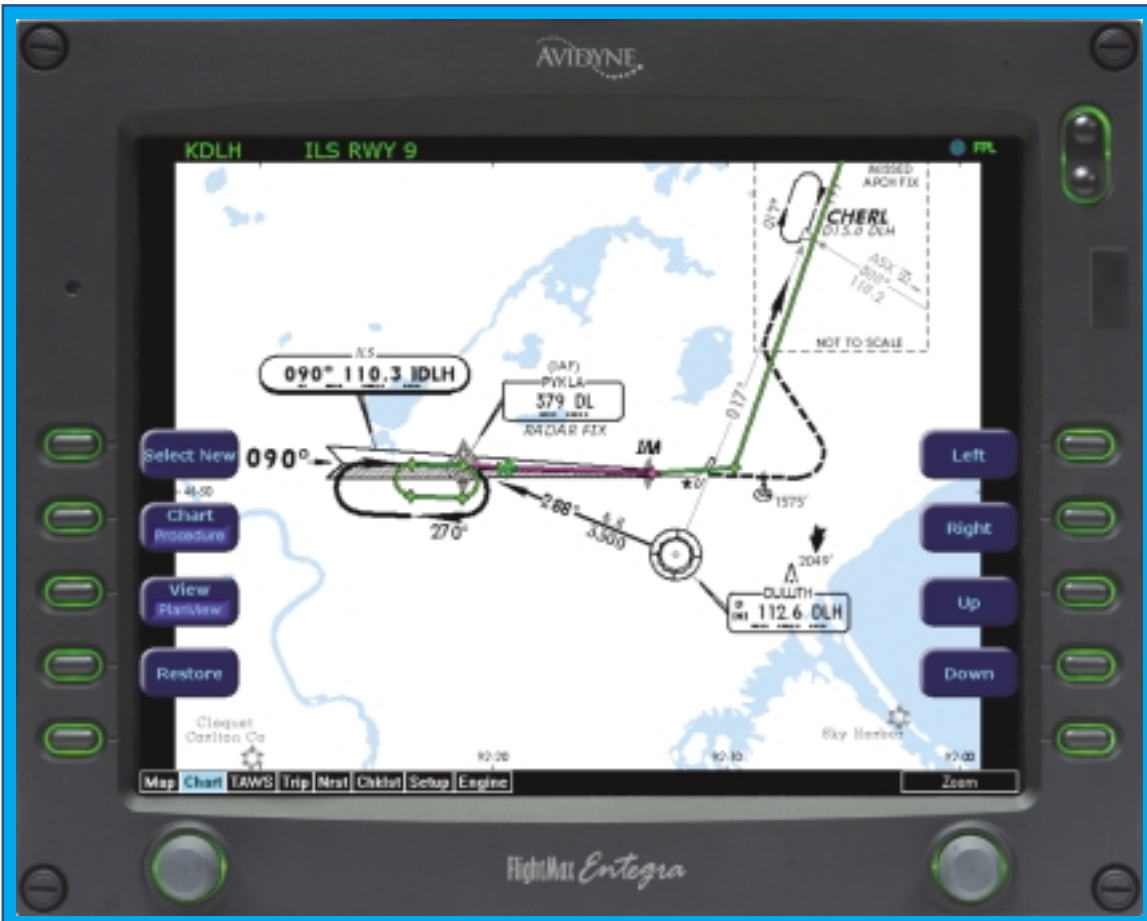
An Avidyne® Multifunction Display (MFD) displays an approach procedure. (Avidyne® photo)
