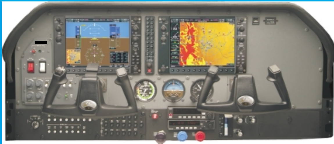
A Cessna 182 cockpit with a Garmin G1000™ flight deck. (Garmin photo)
