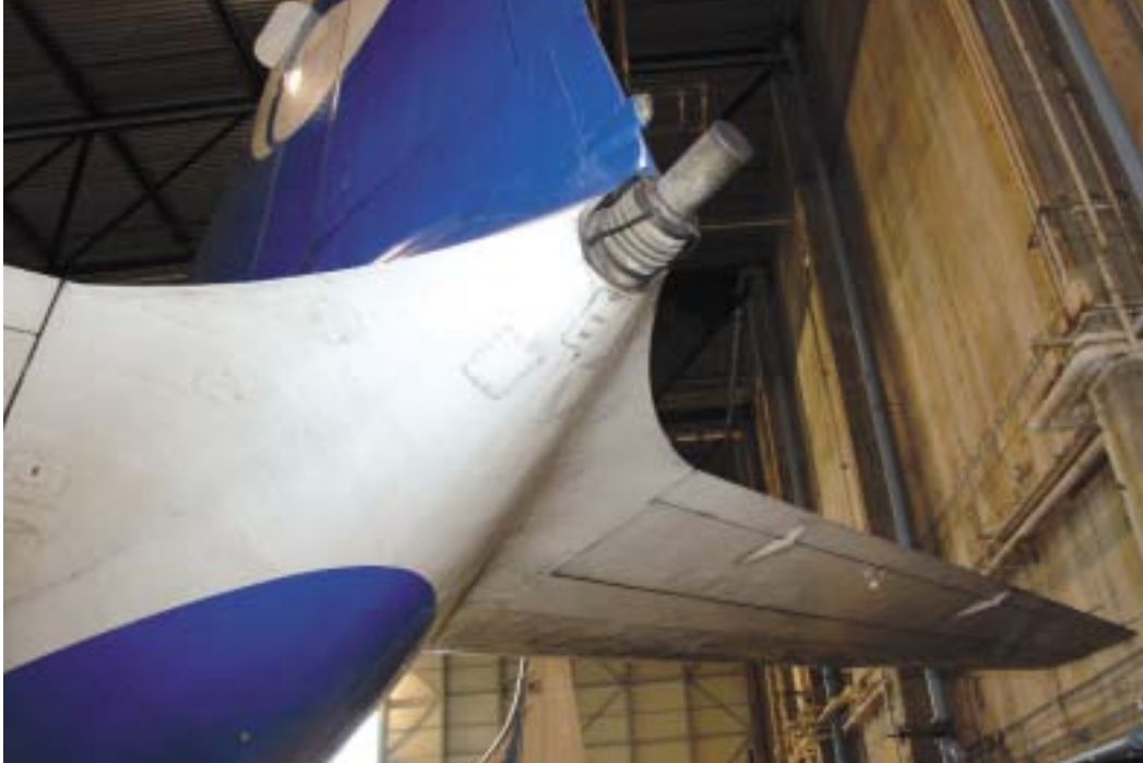
The venerable FAA Convair 580 and the "Hard Point" where the lightning rod was mounted for the thunderstorm research.
