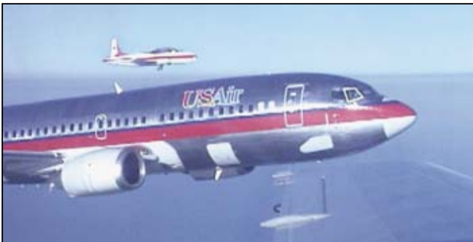
Research was conducted based on a 1994 accident involving a Boeing 737 near Pittsburgh, PA. It was thought that a wake encounter may have initiated the upset event. The T-33 (background) was the photo aircraft. Its speed brakes are extended.
