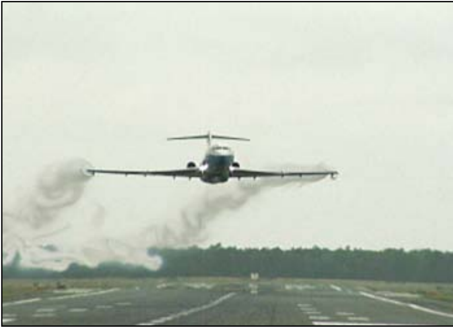
The wingtip smoke generators and (center) the oil tanks, or "kegs" as they're called, containing the oil used for the smoke.
