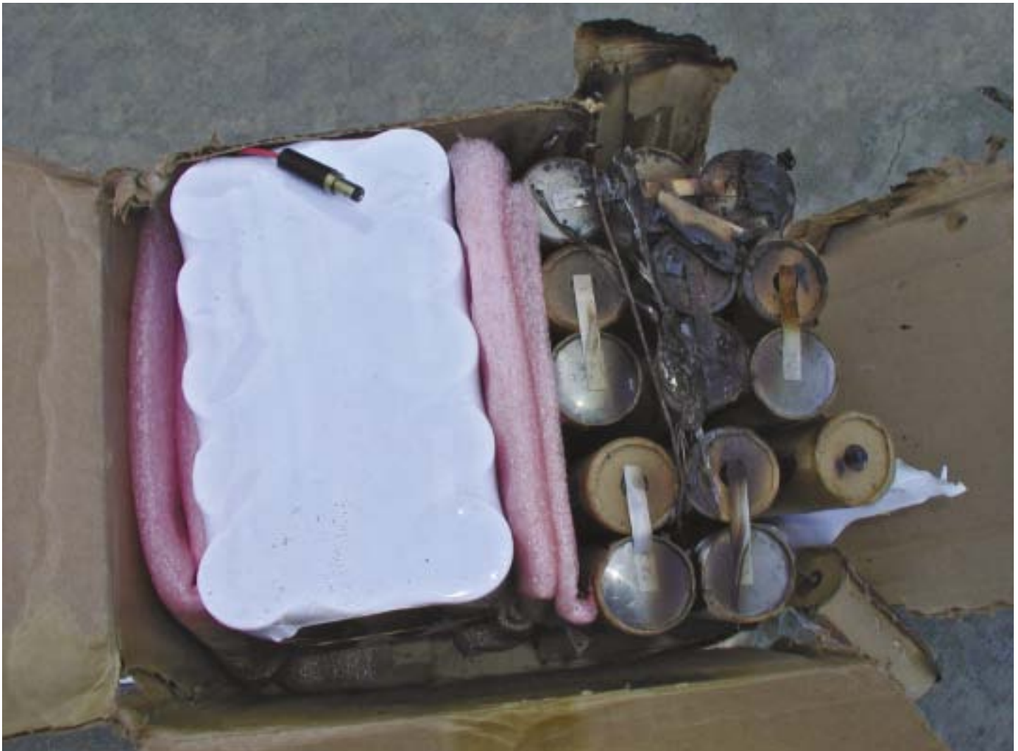
Left photo shows fire damage caused by a burning battery in an air carrier overhead storage bin. Above, a close-up of batteries after a fire.
