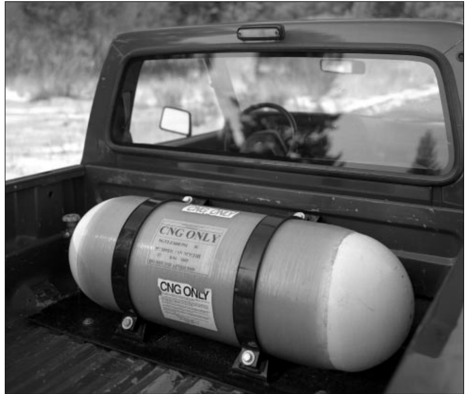
Figure 1. Typical installation of a CNG tank in a pickup
