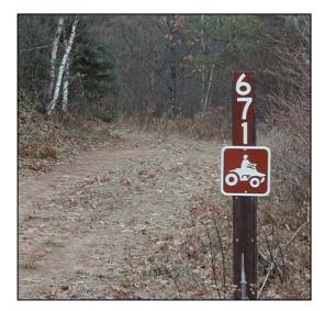
generally to the right of the main intersection with another road, such as a Township Road. The sign is an 8-inch square on a fiberglass post, 4 to 5 feet above the ground. The Forest Road numbers appear above the ATV symbol.
