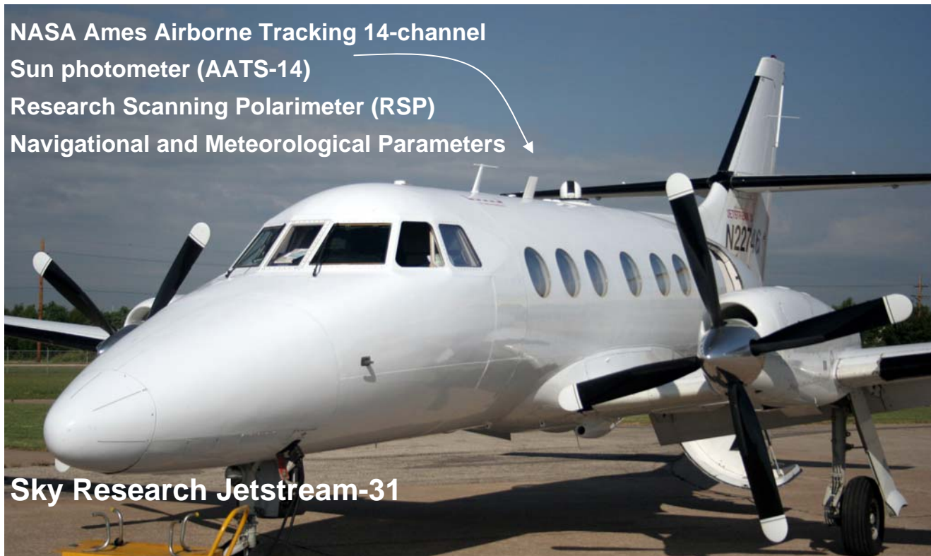
Figure 1. Optical head of AATS-14 mounted external to the J-31 aircraft skin.
