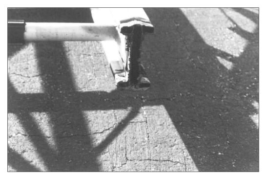
Cross section of the main beam of the Mundelein ladder after it was cut to remove the damaged sections. The beam is assembled from several section of flat steel strips which are bent to form the flanges and then welded together to create the I-beam shape. The interior of the beam is hollow.
