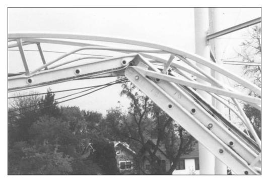
This photo shows a close-up view of the point of failure just above the bed section in the Mundelein incident. Ladder failures often occur at this point in the ladder.
