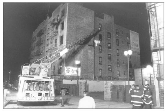
In a recreation of the FDNY Ladder104 collapse scene, Ladder 112 is positioned with its ladder extended to the window where the occupants were trapped. The ladder is extended 91 feet at a 31 degree elevation angle.
