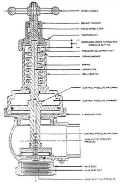
Figure 1 Direct-acting type pressure reducing valve.
