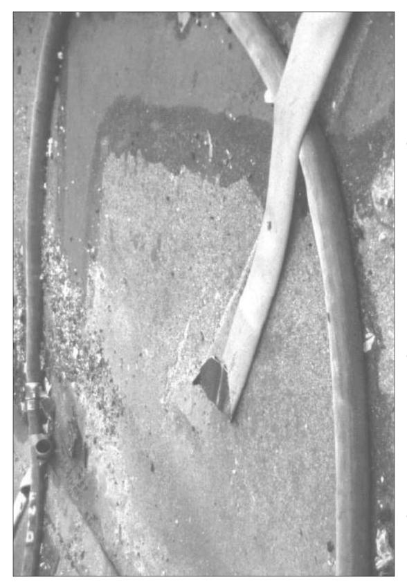
entering the stairways were damaged several times and had to be replaced at great risk to firefighters. (Shoring boards were Section of 5-inch hose that was ruptured by falling debris outside the building. Hose lines feeding the standpipes and later used to protect the hose lines.)
