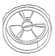
PRESSURE RESTRICTING DEVICE - separate fitting which attaches to the outlet of a standpipe valve. Device is easily removed to obtain full unrestricted flow.
