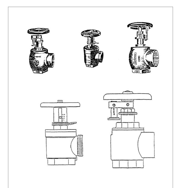
PRESSURE RESTRICTING VALVES - Pressure restricting valves are easily recognizable due to the external fittings on the bonnetts and stems (release links and clips, collars, etc.).
