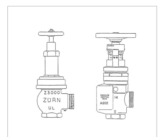
PRESSURE REGULATING VALVES - Direct acting pressure reducing (pressure regulating) valves are required to be permanently marked with: the name or trademark of the manufacturer or private labeler, and a distinctive model number, catalog designation, identification mark, or the equivalent. If unsure whether a particular valve is a PRV, contact the Inspections unit with the above information.
