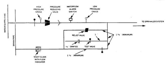
Figure 4. Arrangement of pressure reducing valve for individual sprinkler systems. typically seen on each floor of a high-rise building.
