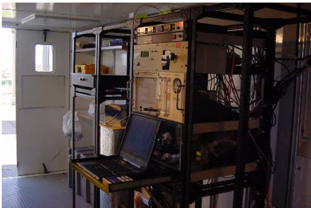
Figure 4. The AOS instrument and rack system inside the Aerosol Trailer at Point Reyes.
