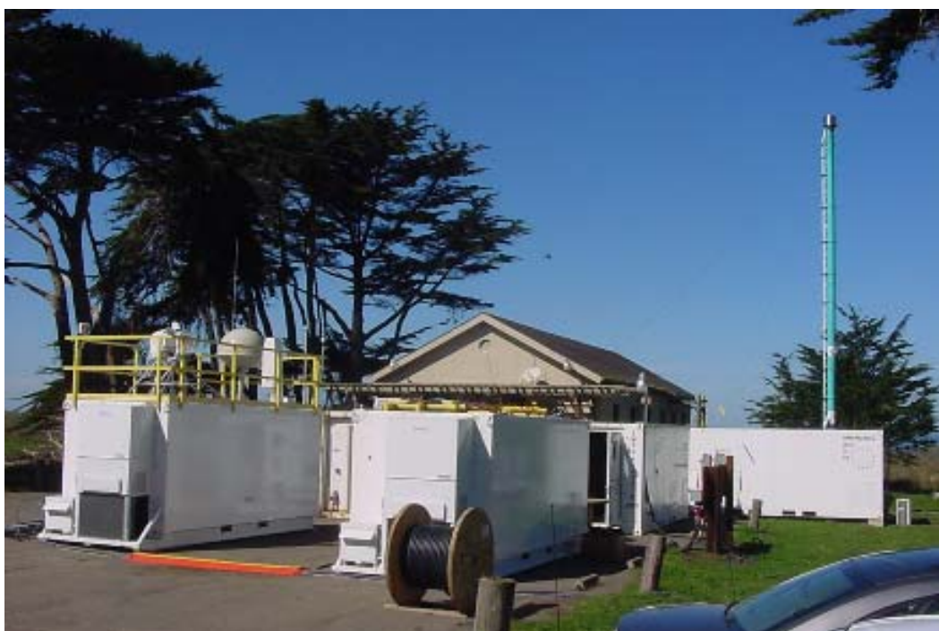
Figure 3. Trailers of the ARM Mobile Facility deployed at Point Reyes, California, in 2005. The Aerosol Trailer and aerosol sampling stack are visible at the right side of the photograph.
