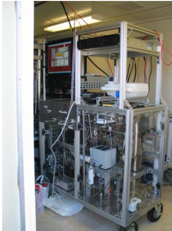
Figure 2. The HTDMA system that was installed in the SGP Aerosol Trailer in 2005.
