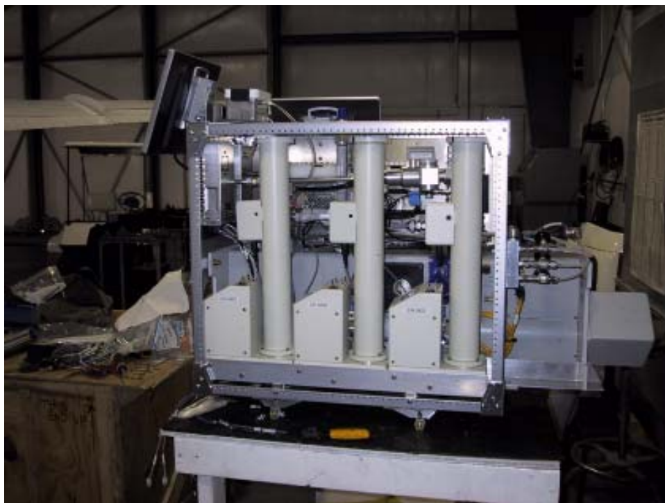
Figure 7. The IAP Aerosol Optics rack for improved aerosol hygroscopic growth measurements.
