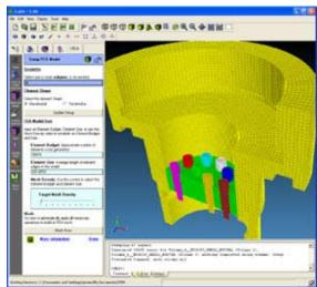
An example of ITEM used to mesh a CAD model representing a weapon component. Left: ITEM detects and previews an option for decomposing the model for hexahedral mesh. Right: The final hexahedral mesh after using ITEM to help prepare the CAD model.
