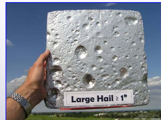
Aluminum foil-wrapped Styrofoam hail pads
