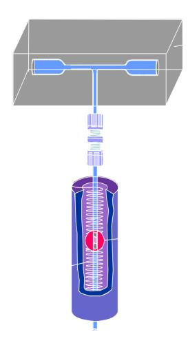
This apparatus was designed to study the thermal desorption of mercury and mercury compounds from CCBs at temperatures from ambient to 700°C.
