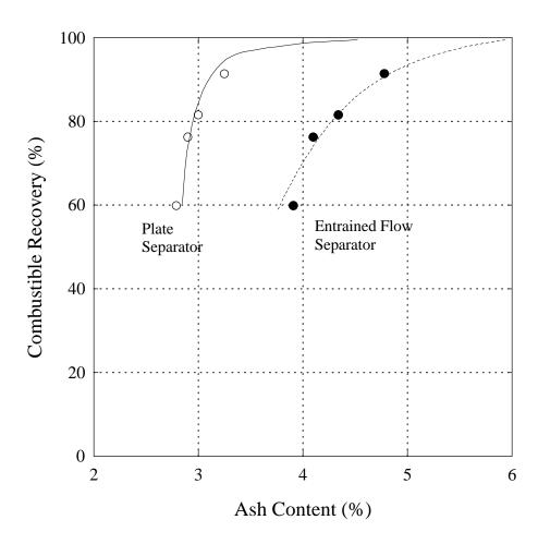
Figure 7. Product ash content as a function of combustible recovery. The results were obtained on Pittsburgh No. 8 clean coal sample in the TES bench-scale Unit separation study.
