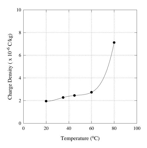
Figure 4. Effect of temperature on charge density. The results were obtained on Pittsburgh No. 8 coal sample with a 200 g/min feed rate.
