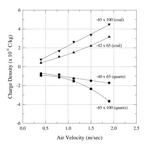
Figure 2. Effect of air velocity on charge density using Pittsburgh No.8 clean coal sample and quartz with a variety of particles sizes.
