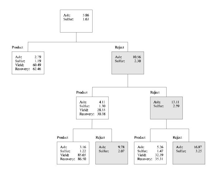
Figure 6. Separation test flowsheet for the bench-scale TES unit. The results were obtained with a Pittsburgh No.8 clean coal sample at electrode potential of 70 kV. Assays for each of the test were measured from the sample scraped from the drum electrodes.
