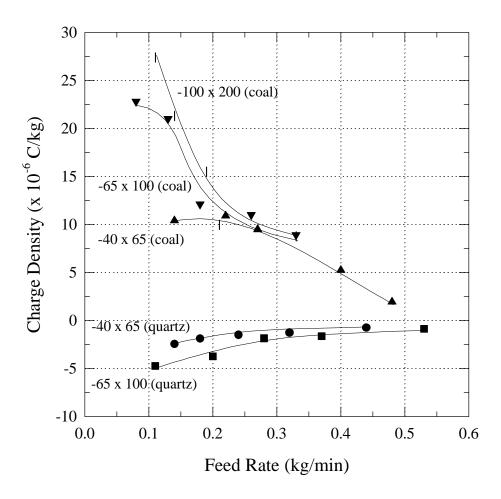
Figure 3. Effect of particle feed rate on charge density using Pittsburgh No.8 clean coal and quartz samples with a variety of particle size.
