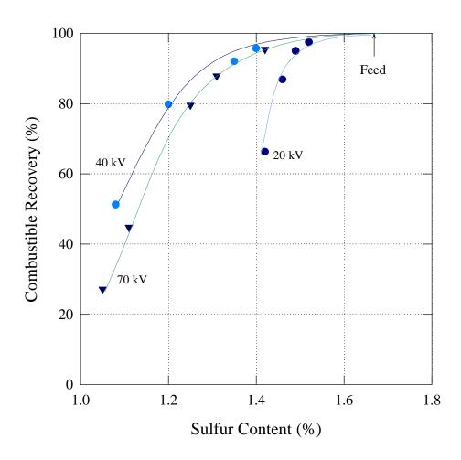
Figure 10. Grade vs. Recovery curves of the bench-scale TES unit. The results were obtained on -200 mesh Pittsburgh No. 8 clean coal samples with 20, 40, and 70 kV electrode potential settings
