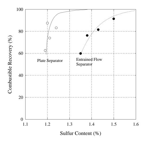
Figure 8. Product sulfur content as a function of combustible recovery. The results were obtained on Pittsburgh No. 8 clean coal sample in the TES bench-scale Unit separation study
