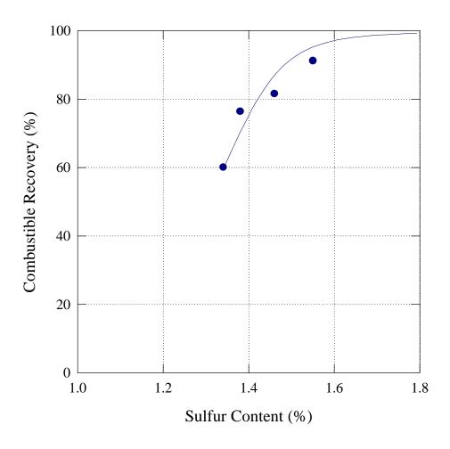
Figure 12. Grade (sulfur content) vs. Recovery curve of the bench-scale TES unit. The results were obtained on -140+200 mesh Pittsburgh No. 8 clean coal samples with electrode potential at  $70~\rm kV$
