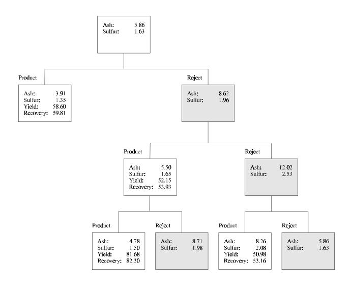
Figure 5. Separation test flowsheet for the bench-scale TES unit. The results were obtained with a Pittsburgh No.8 clean coal sample at electrode potential of 70 kV. Assays for each of the test were measured from the bulk sample.
