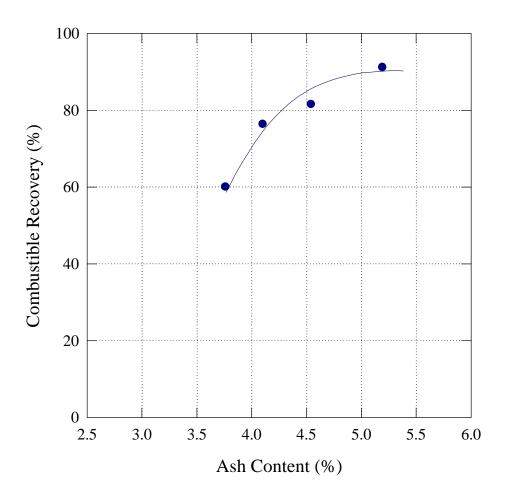
Figure 11. Grade vs. Recovery curve of the bench-scale TES unit. The results were obtained on -140+200 mesh Pittsburgh No. 8 clean coal samples with a 70kV electrode potential
