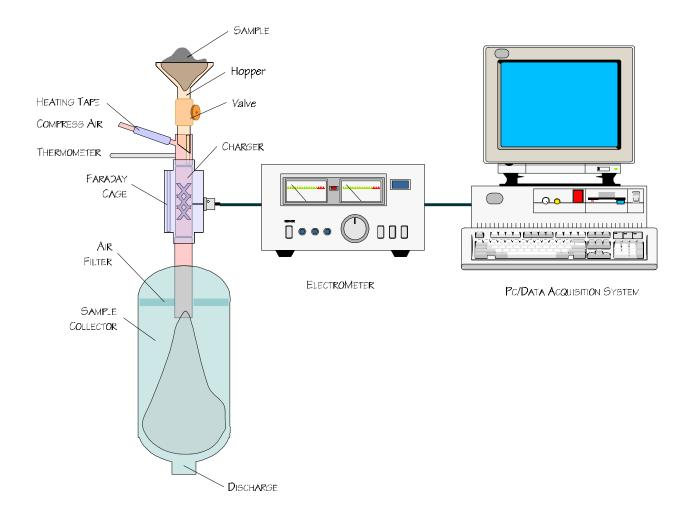
Figure 1. Schematic representation of the on-line charge measurement device with heating system and temperature sensor for studying tribocharging mechanism used in the present work.
