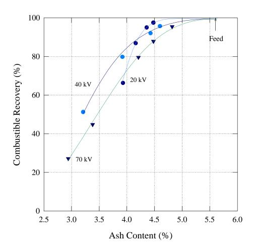
Figure 9. Grade vs. Recovery curves of the bench-scale TES unit. The results were obtained on -200 mesh Pittsburgh No. 8 clean coal samples with 20, 40, and 70 kV electrode potential settings.
