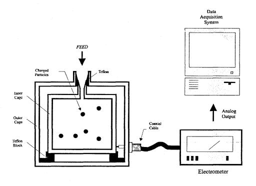
Figure 2. Instrumentation setup for the particle charge measurement using a Faraday cage.
