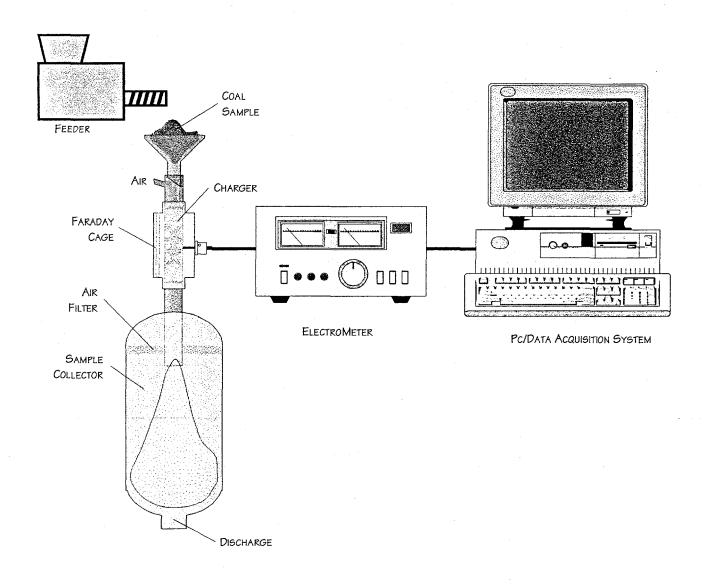
Figure 5. Schematic representation of charge measurement setup using the on-line charge measurement device.
