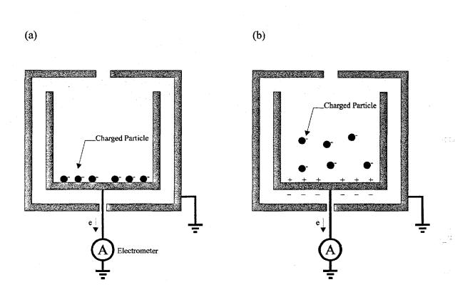
Figure 3. Schematic representation of the principles of particle charge measurement using a Faraday cage
