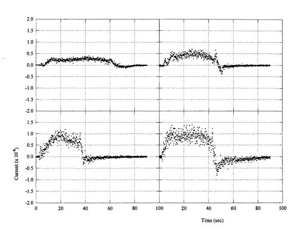
Figure 6. A printout from the data acquisition system used in conjunction with the on-line charge measurement device. The results were obtained on a Pittsburgh No. 8 coal sample (-28x 65 mesh) with different aeration rates.
