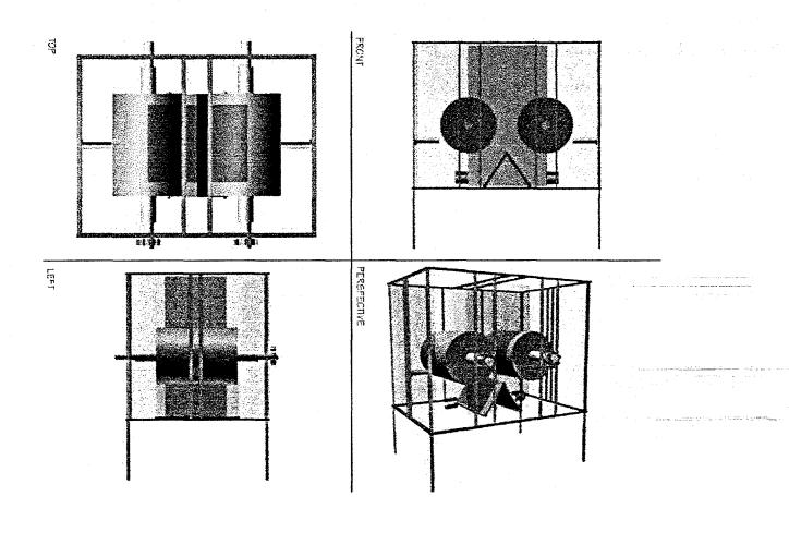
Figure 13. Schematic representation of the modified engineering design of the open-gradient triboelectrostatic separator used in the present work
