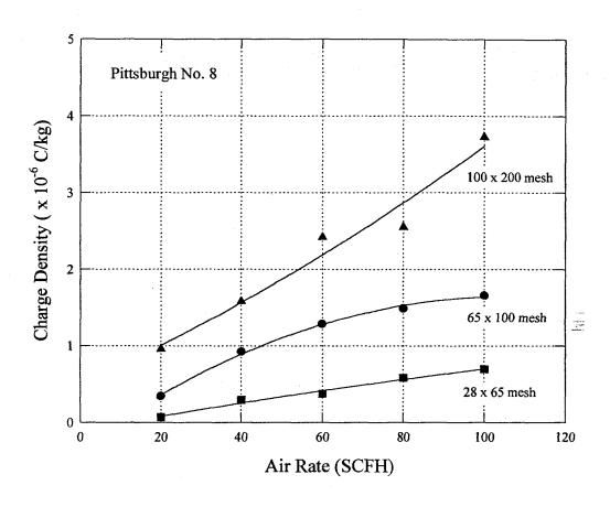
Figure 7. Effect of aeration rate on charge density. The results were obtained on Pittsburgh No. 8 coal samples with different particle size.
