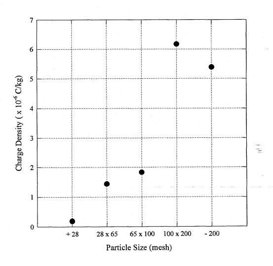
Figure 9. Effect of particle size on charge density. The results were obtained on Pittsburgh No. 8 coal samples with a 150 g/min feed rate.
