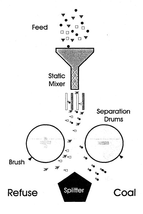
Figure 10. Schematic representation of the open-gradient triboelectrostatic separator used in the present work.
