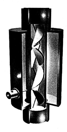
Figure 4. Schematic representation of the on-line charge measurement device for studying triboelectrification used in the present work.
