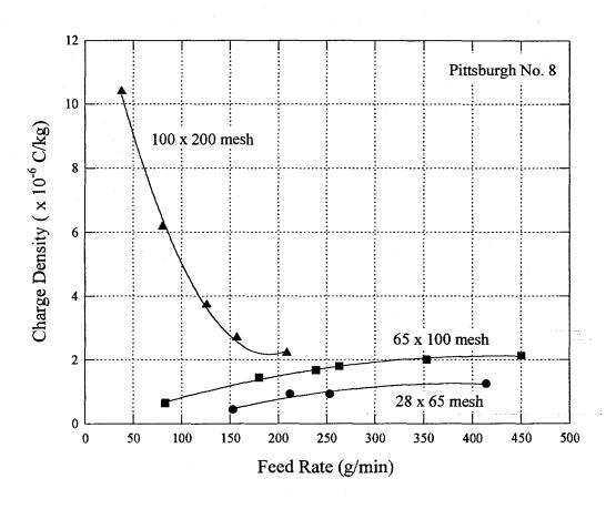
Figure 8. Effect of feed rate on charge density. The results were obtained on Pittsburgh No. 8 coal samples with different particle size.
