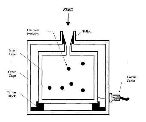
Figure 1. Schematic representation of the Faraday cage used in the present work.
