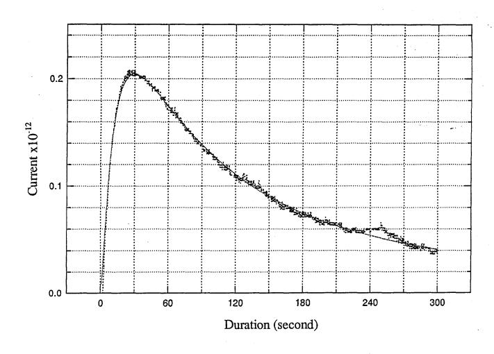
Figure 6. A printout from the data acquisition system used in conjuction with the Faraday cage. The result was obtained with a Pittsburgh No. 8 coal sample (-65 x 100 mesh)
