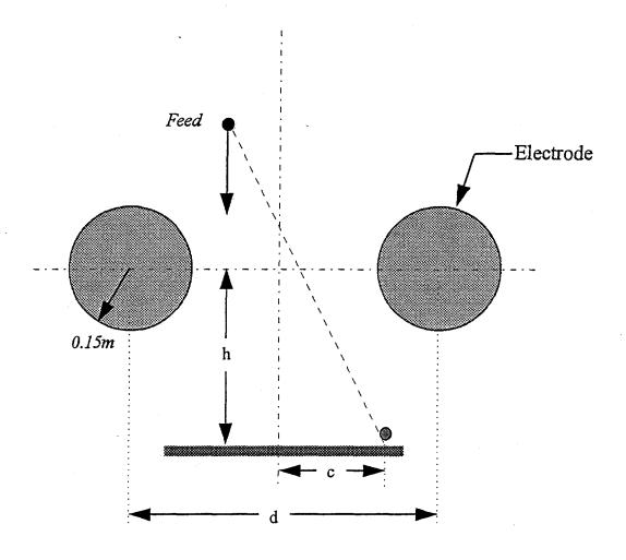
Figure 10. Movement of a charged particle in a non-uniform electric field created by cylindrical electrodes; a and b represent the original position, c represents deflection of the particle on the collection plate, and d represents the distance between the centers of the electrodes
