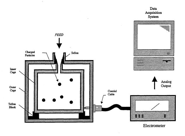
Figure 3. Instrumentation for the particle charge measurement using a Faraday cage
