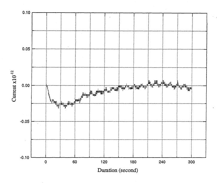
Figure 4. A printout from the data acquisition system used in conjuction with the Faraday cage. The result was obtained with a quartz sample ( $60\mu m$ )
