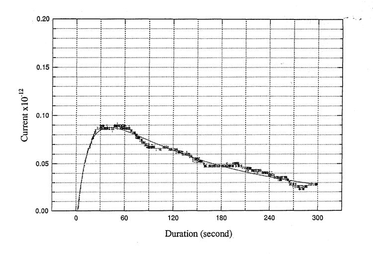
Figure 5. A printout from the data acquisition system used in conjuction with the Faraday cage. The result was obtained with a Pittsburgh No. 8 coal sample (+65 mesh)
