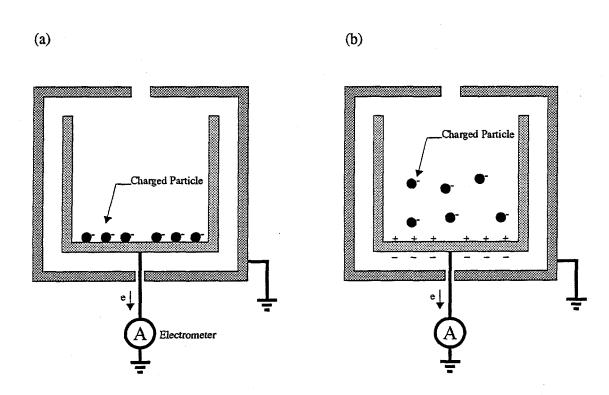
Figure 1. Schematic representation of the principles of particle charge measurement using a Faraday cage
