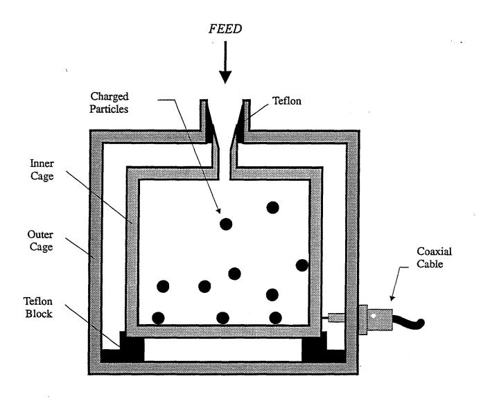
Figure 2. Schematic representation of the Faraday cage used in the present work
