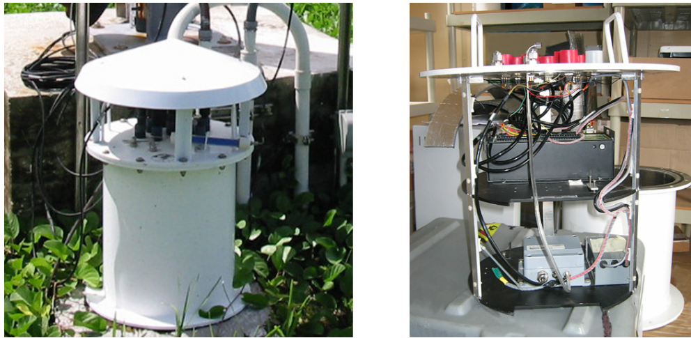
Figure 1. Aluminum canister housing installed at a TWP field site (left), and the canister housing disassembled to reveal the ZENO ® 3200 data logger (black box) and internal wiring (right).
