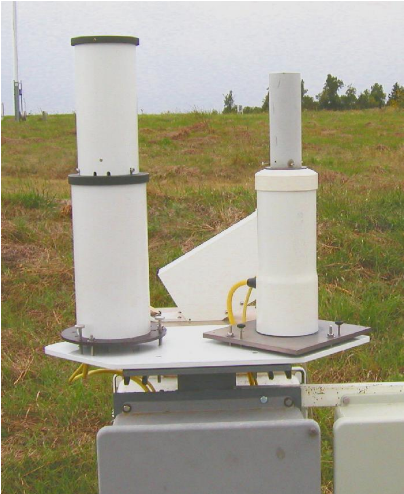
Figure 3d. The single-channel and two-channel NFOV instruments.
