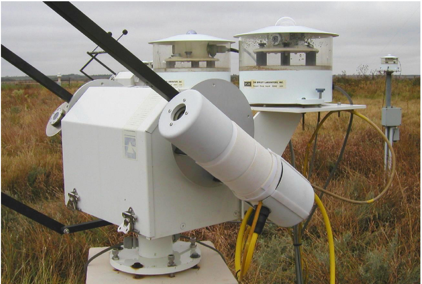
Figure 3. Photos of the various MFRSR-derived instruments. Figure 3a shows the NIMFR that is located at the SGP Central Facility. This instrument is located on the EF-13 solar tracker.
