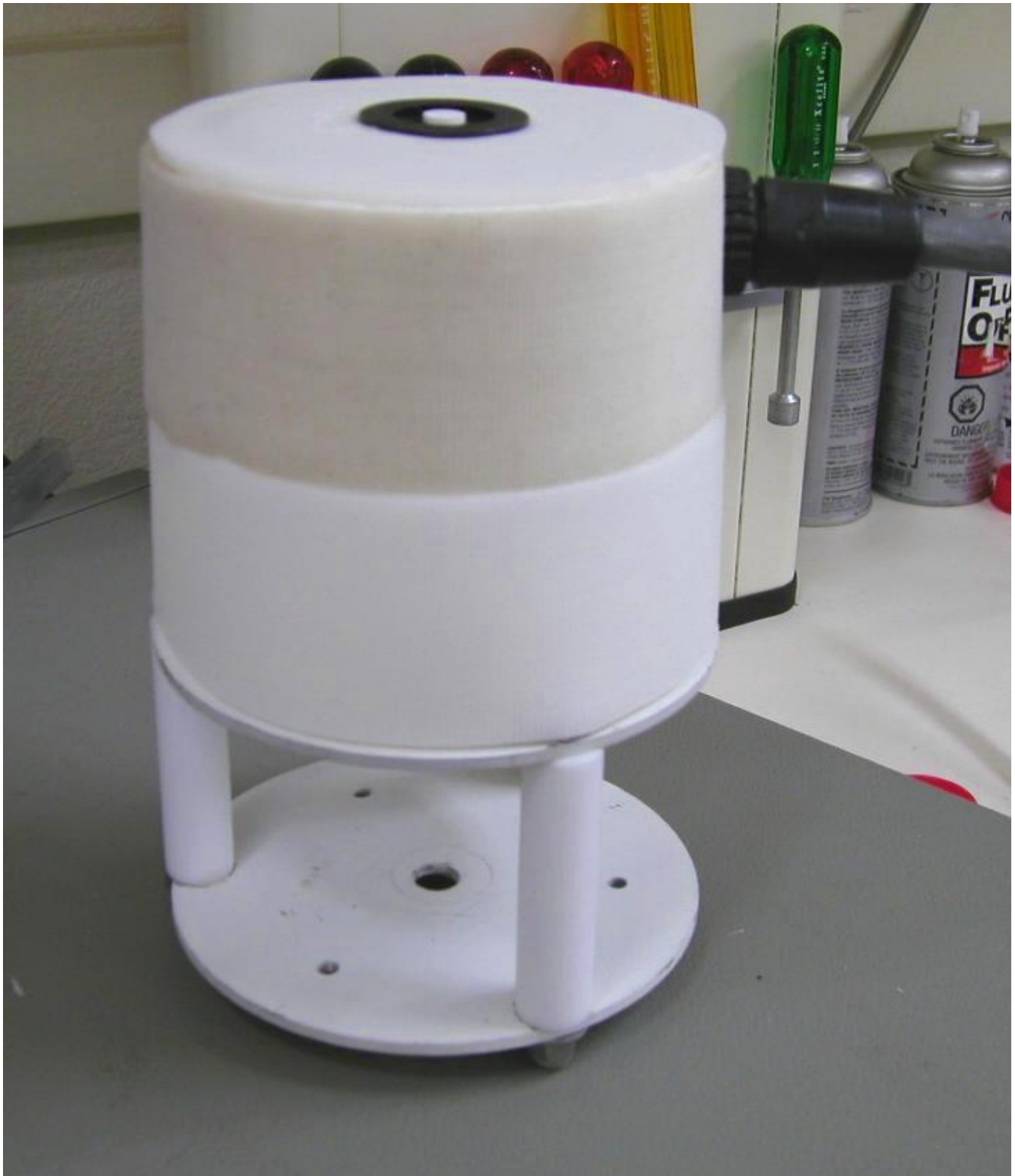
Figure 3c. An MFR contained in an insulated housing required for deployments in the NSA.
