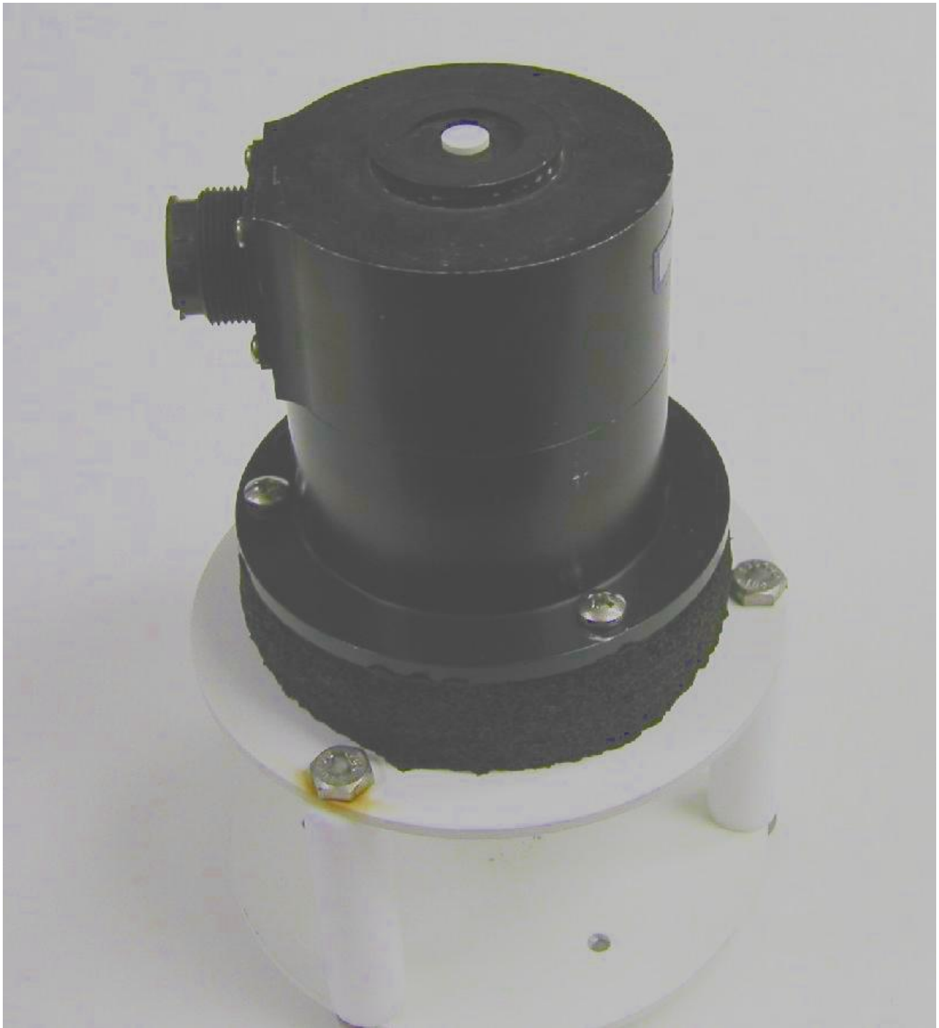
Figure 3b. An MFR – this instrument is mounted on towers pointed at the surface to provide data on reflected irradiances.
