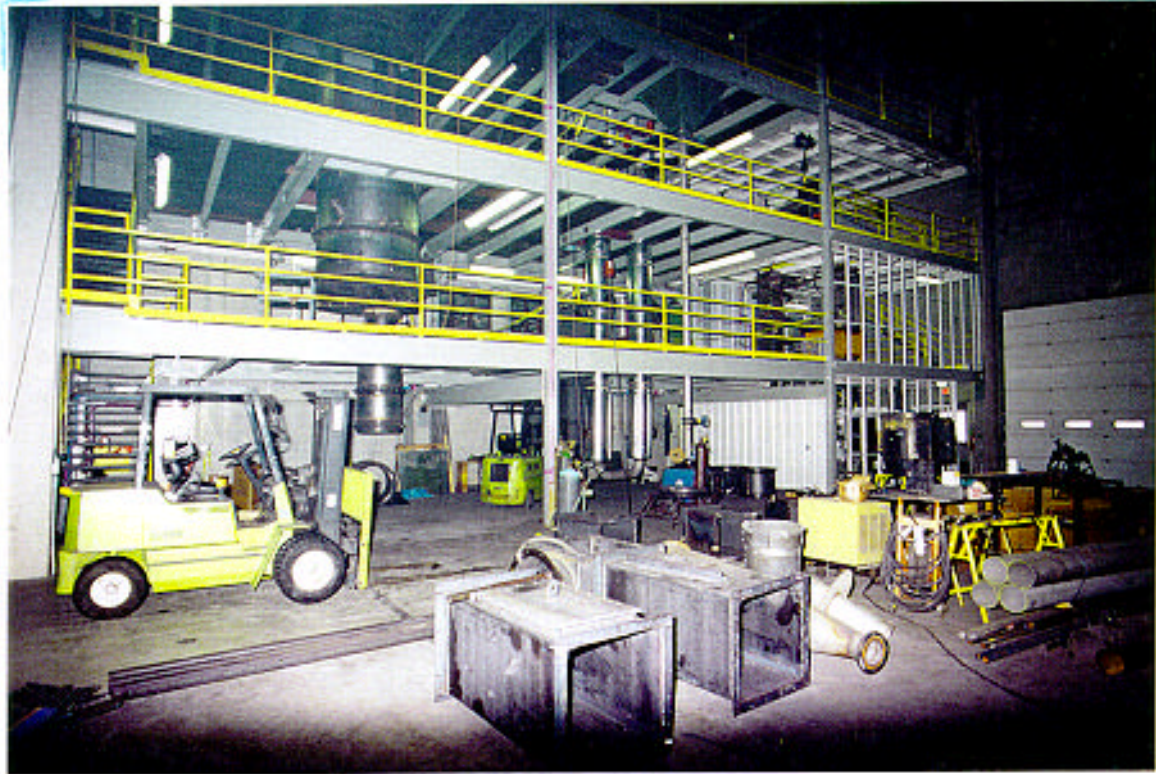
Exhibit 2.2-14 Photograph Showing Furnace Slag Pot Shell Sections In The Background And The CAH Shell Sections In The Foreground
