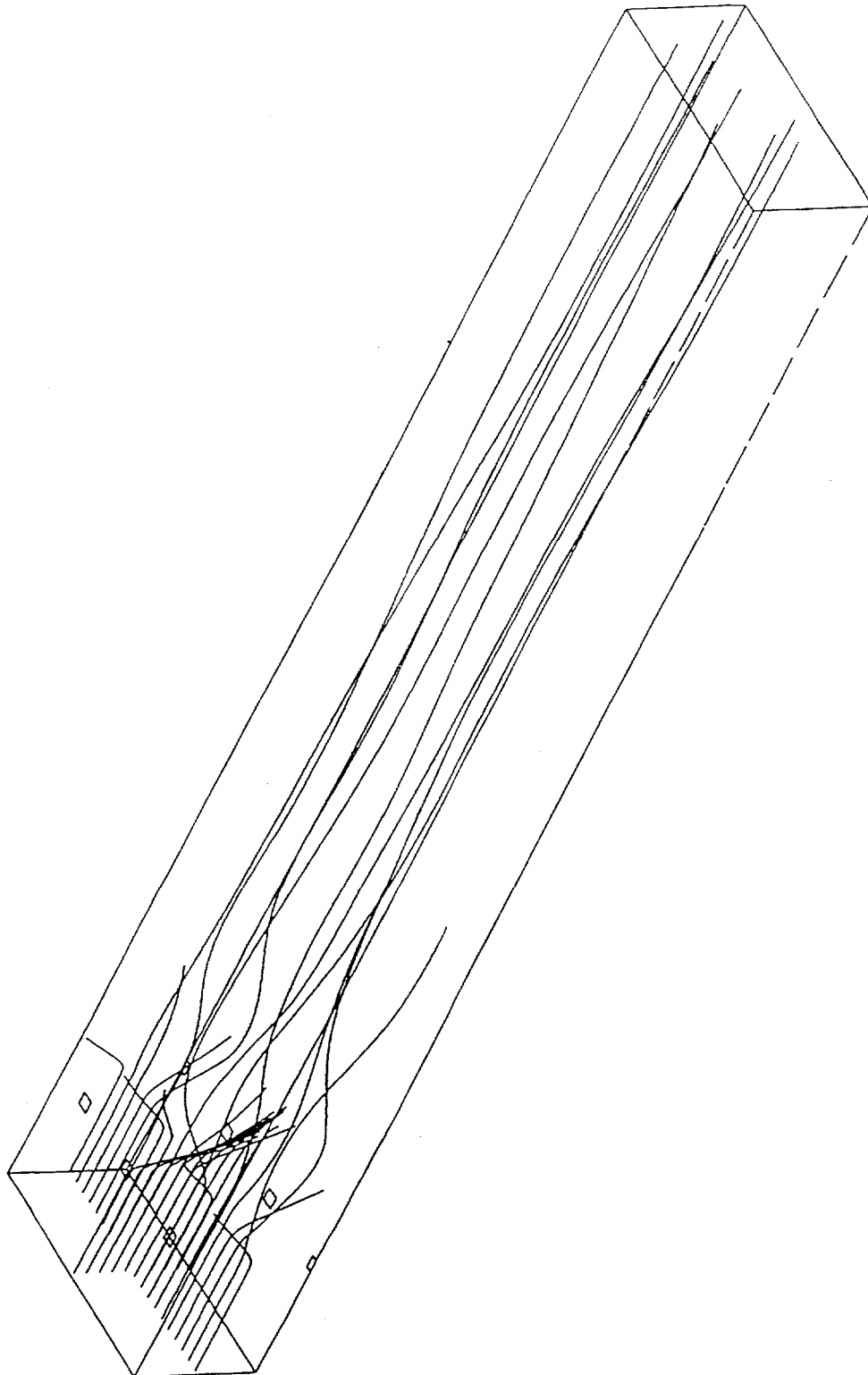
Selected Trajectories for Quench 6 Case with 30-Micron Diameter Particles Exhibit 2.3-53
