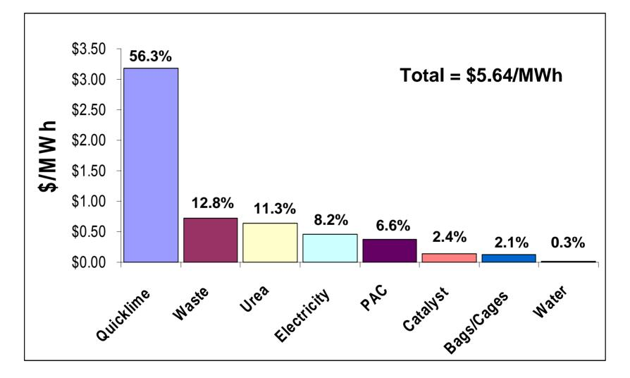
Assumptions: SNCR NSR = 1.50, catalyst life = 3 yr, Ca/S molar ratio (inlet  $SO_2$ ) = 1.55, CaO purity = 95% (w/w), PAC feed rate = 3.5 lb/MMacf, baghouse bag / cage life = 5 yr
