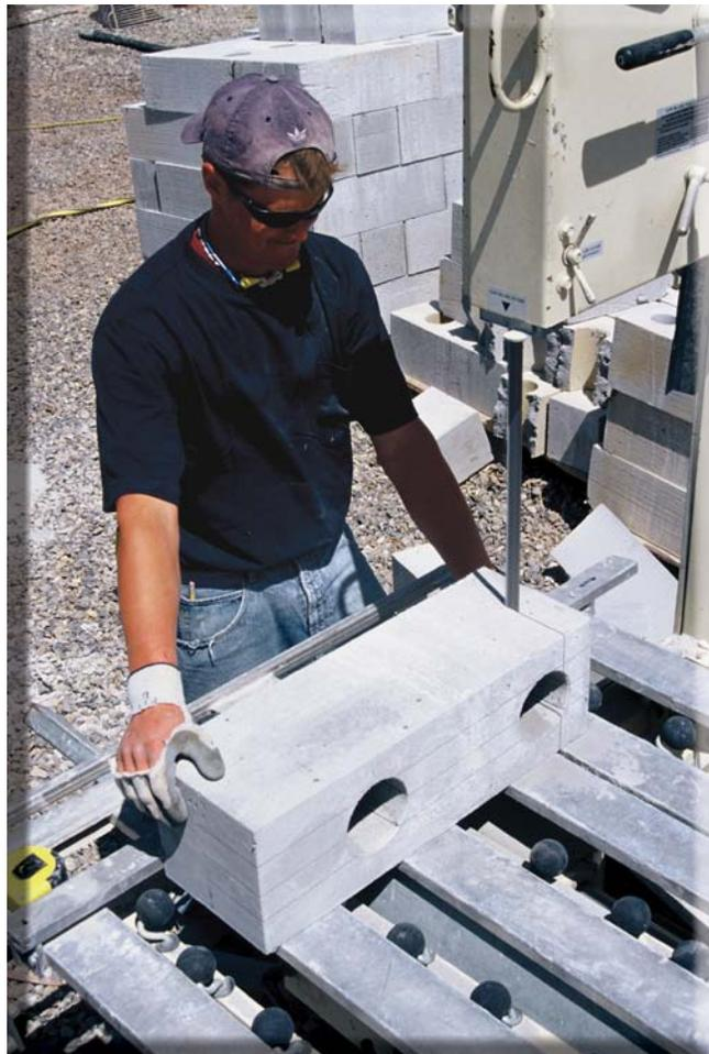
Light-weight concrete block made with CUBs.
