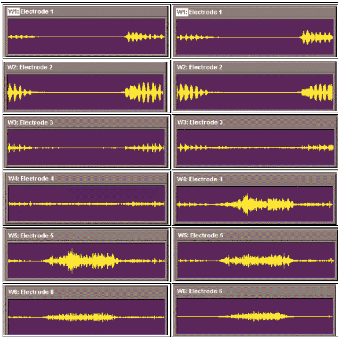
Figure 10a & 10b Processor response to male token input /sh/, 1 st exemplar, using scale x:376-716, y: \pm 4.9 for both.
