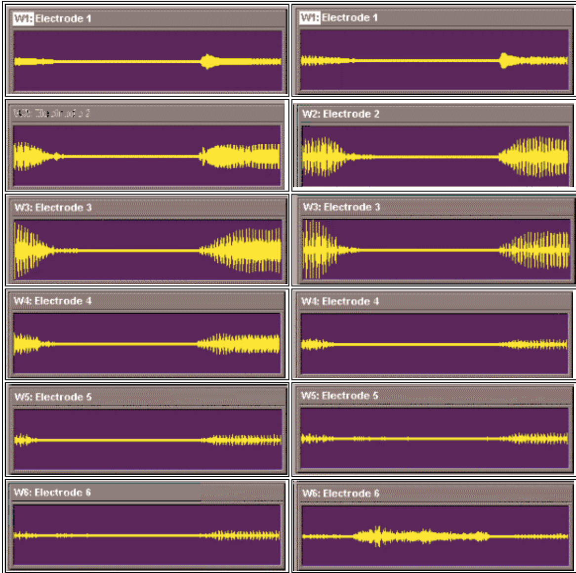
Figure 1a & 1b Processor response to female token input /s/, 1 st exemplar, using scale x:480-840, y: \pm 2.9 for both. Part a (left) is for a processor spanning the frequency range 350-5500Hz, while b is for a processor spanning the frequency range 350-9500Hz.
