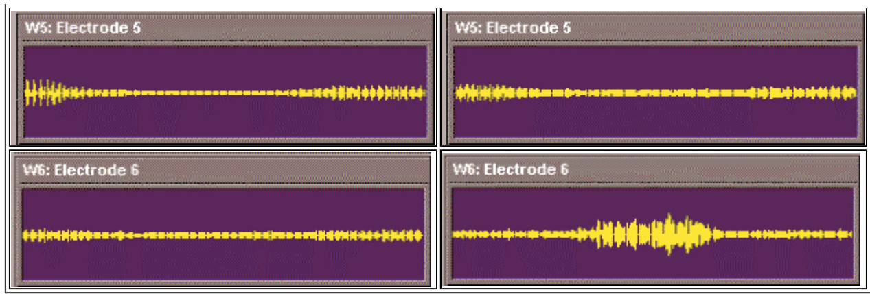
Figure 3a & 3b Processor response to female token input /z/, 1 st exemplar, using scale x:460-760, y: \pm 2.9 for both. Part a (left) is for a 350-5500Hz processor and b for a 350-9500Hz processor.
