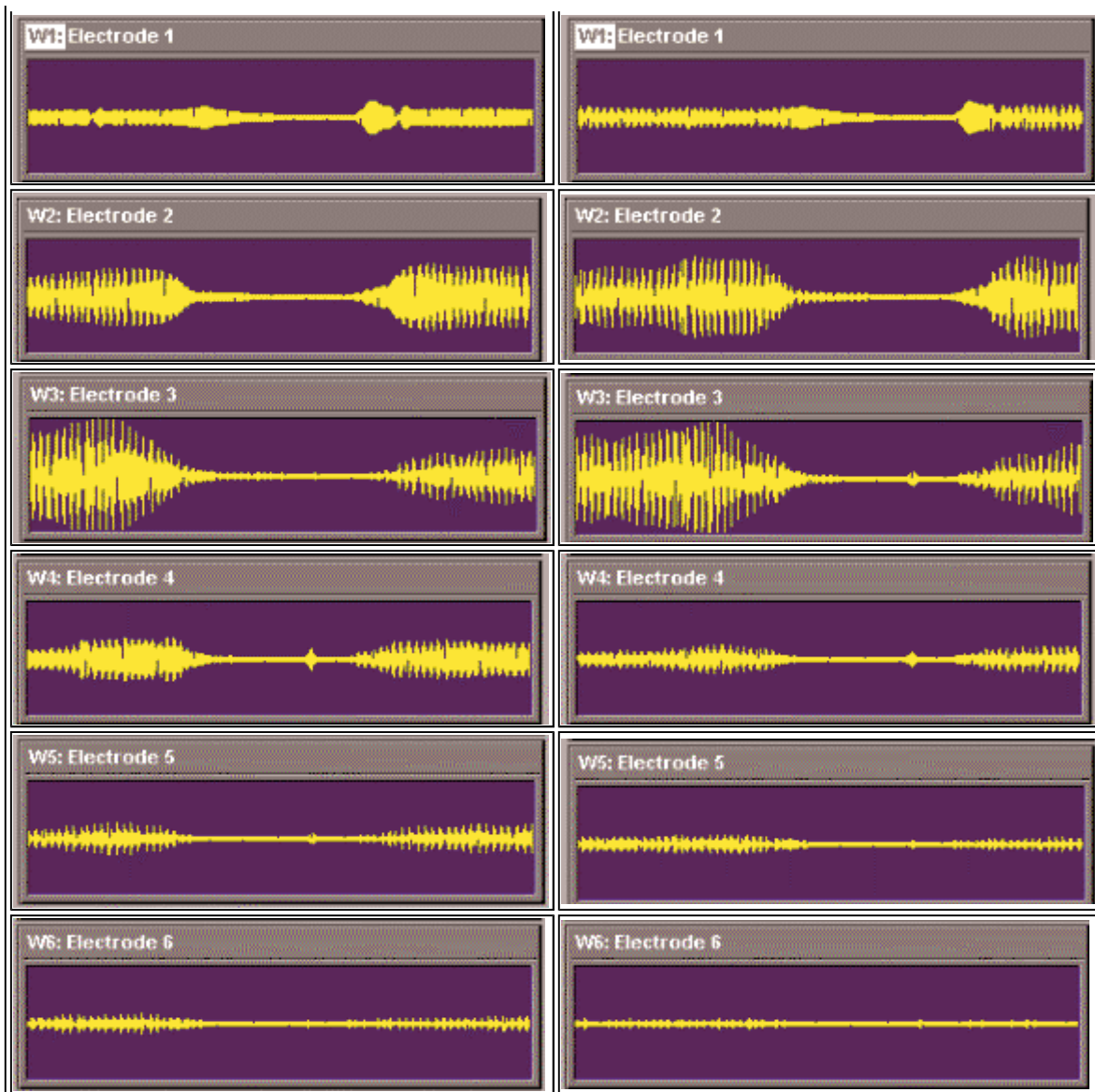
Figure 5a & 5b Processor response to female token input /g/, 1 st exemplar, using scale x:480-780, y: \pm 2.9 for both. Part a (left) is for a 350-5500Hz processor and b for a 350-9500Hz processor. Notice how the energy from channel 4 in the narrow range processor gets distributed between channels 3 and 4 in the expanded frequency processor. Also channel 1 here looks more distinct than channel 1 in the expanded version.
