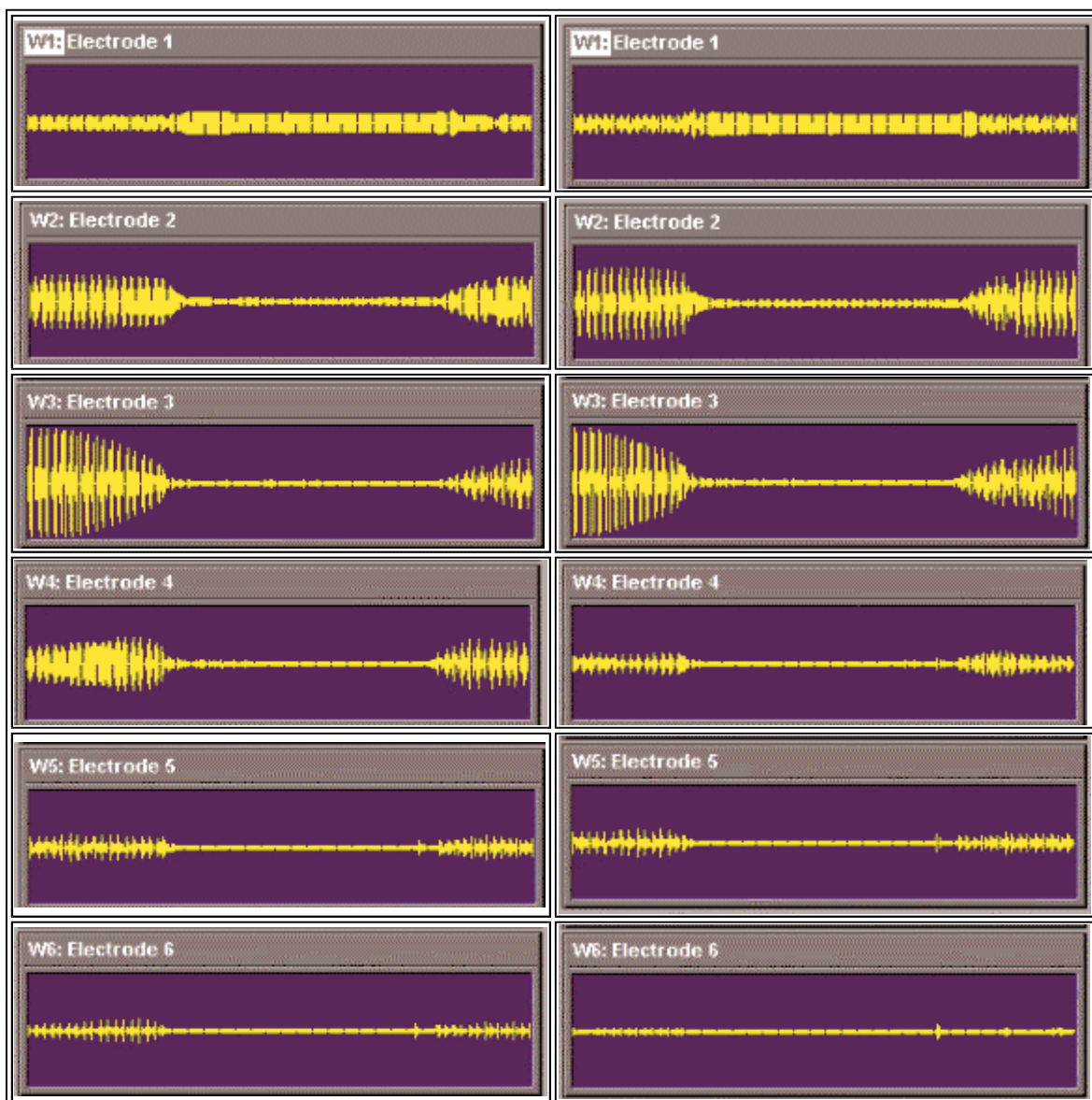
Figure 7a & 7b Processor response to female token input /n/, 1 st exemplar, using scale x:460-740, y: \pm 2.9 for both. Part
