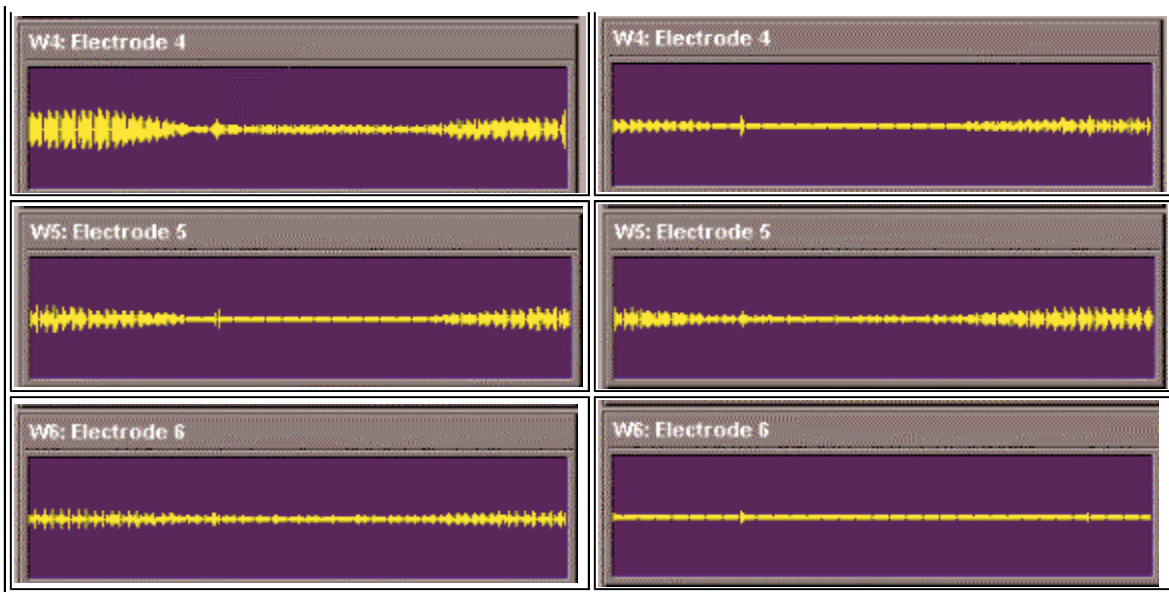
Figure 6a & 6b Processor response to female token input /m/, 1 st exemplar, using scale x:460-740, y: \pm 2.9 for both. Part a (left) is for a 350-5500Hz processor and b for a 350-9500Hz processor.
