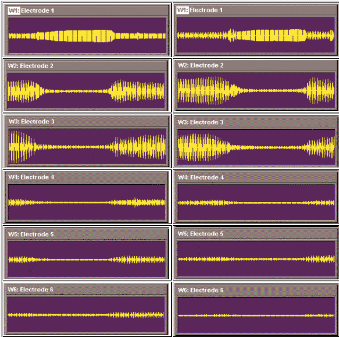
Figure 8a & 8b Processor response to female token input /l/, 1 st exemplar, using scale x:460-740, y: \pm 2.9 for both. Part a (left) is for a 350-5500Hz processor and b for a 350-9500Hz processor.
