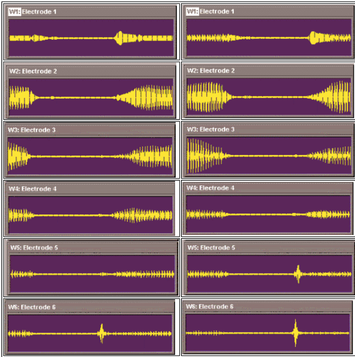
Figure 4a & 4b Processor response to female token input /d/, 1 st exemplar, using scale x:480-780, y: \pm 2.9 for both. Part a (left) is for a 350-5500Hz processor and b for a 350-9500Hz processor.
