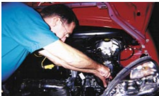
ORNL researcher Brian West installs hardware for emissions tests on the Mercedes A170 diesel vehicle.
