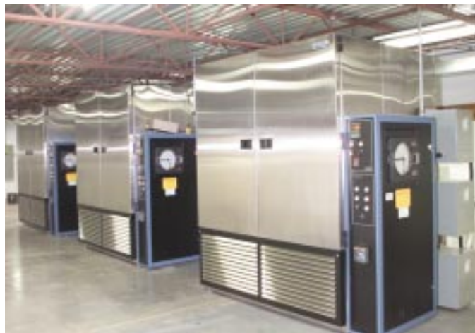
The BTC's Hygrothermal Properties Laboratory will be used to measure the moisture properties of materials typically used in wall systems in Seattle.
