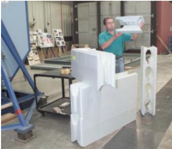
BTC research technician Jerry Atchley examines polystyrene modules of a concrete form wall system used in the Habitat houses.
