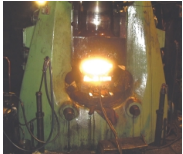
Infrared insert heater preheating dies at Komtek, in Worcester, MA, prior to their use to forge medical hip implants.
