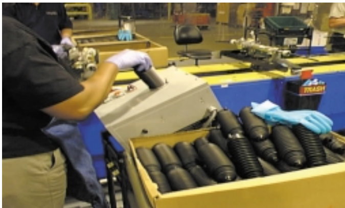
Infrared boot heater being used at Delphi Automotive.
