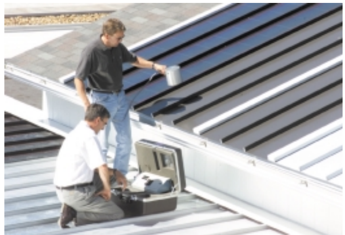
BTC researchers Bill Miller (kneeling) and Jerry Atchley measure the solar reflectance (percentage of solar energy in the visible range that is reflected) of residential roofing systems on a test building at ORNL.
