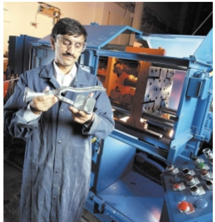
ORNL research scientist Srinath Viswanathan examines a motor mount produced by metal compression forming.
