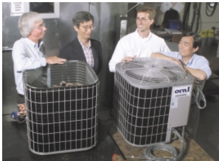
The frostless heat pump developed by BTC researchers (from left) Rick Murphy, Fang Chen, Ron Domitrovic, and Vince Mei eliminates most heat pump defrosting cycles.
