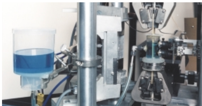
A composite specimen, mounted in the grips of a test machine, undergoes cyclic fatigue loading while immersed in windshield washer fluid (an extreme condition). This is one of a battery of tests imposed on candidate composites.
