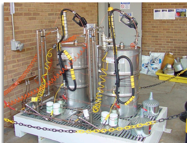
Test units being used to obtain data about E85 and E25 fuel dispensers for Underwriters Laboratories.
