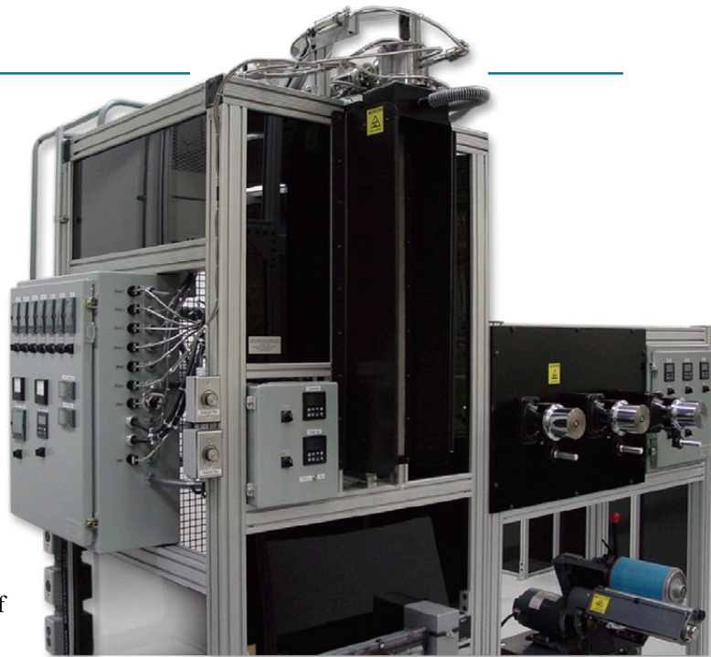
ORNL's multifilament melt spinning equipment.
