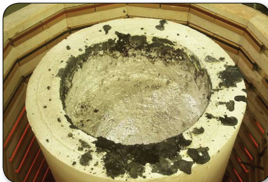
Vessel used in industrial trial at Energy Industries of Ohio. TCON plates are embedded in castable bonite.
