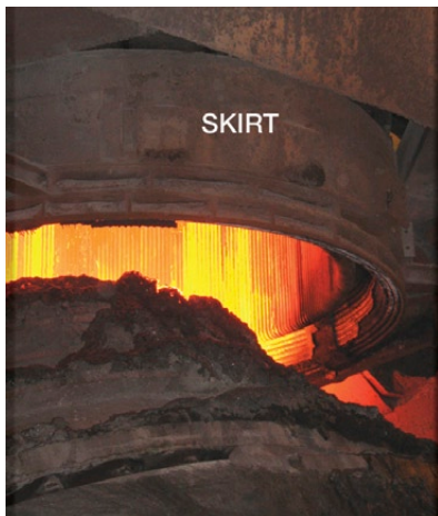
Skirts made of aluminum bronze outlast conventional carbon steel skirts.
