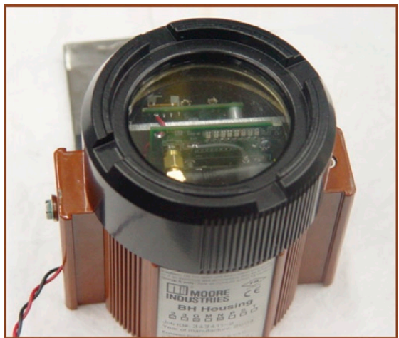
Shock sensor module with wireless communication enclosed in explosion-proof housing.
