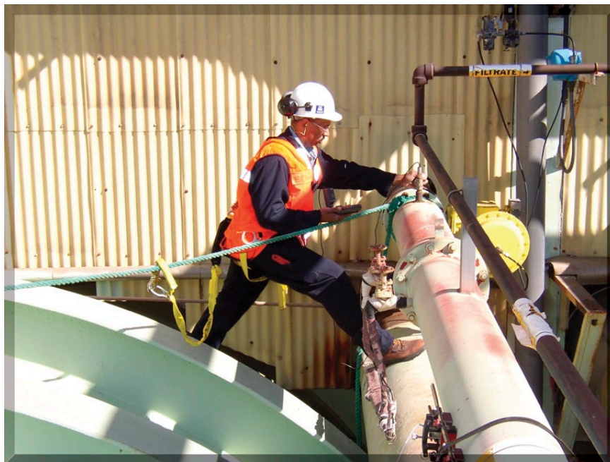
Daryl Cox of ORNL scales a tank to obtain a pressure measurement for a pump discharge as part of an energy efficiency assessment at a paper mill.
