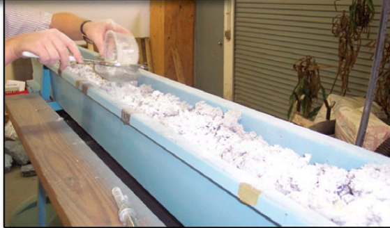
Using a pilot-scale production line (top) different cellulose-PCM blends (bottom) were produced at AFT. ORNL determined that cellulose with 30% added PCM maintains its thermal conductivity.
