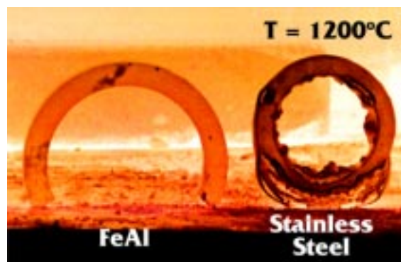
FeAl resists oxidation at high temperatures.
