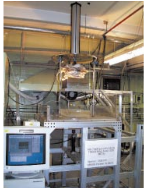
The melt-water explosion triggering analyzer developed at ORNL.
