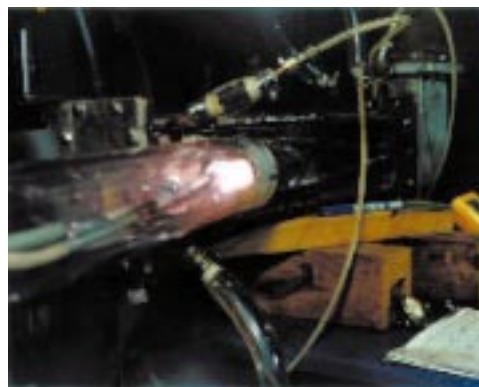
Processing of carbon fibers using microwave plasma (1500°C or greater).
