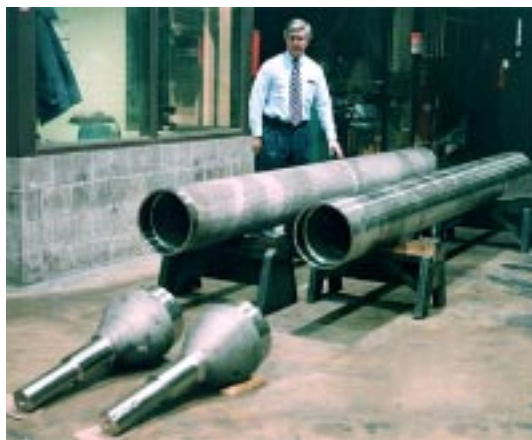
Prototype nickel aluminide transfer rolls for steel mill before installation.
