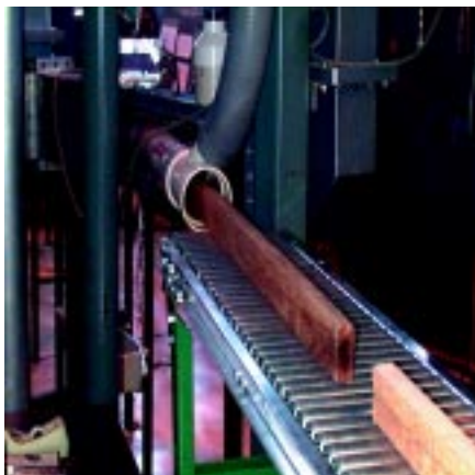
Lumber undergoing microwave drying at ORNL.
