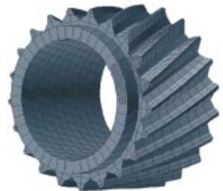
Meshed shape used to simulate a helical gear.
